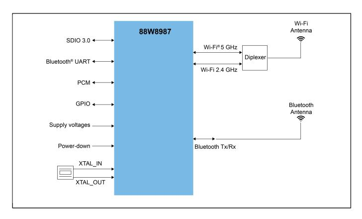
View additional information for 88W8987 (Automotive): 2.4/5 GHz Dual-Band 1x1 Wi-Fi® 5 (802.11ac) + Bluetooth® 5.2 Solution.
