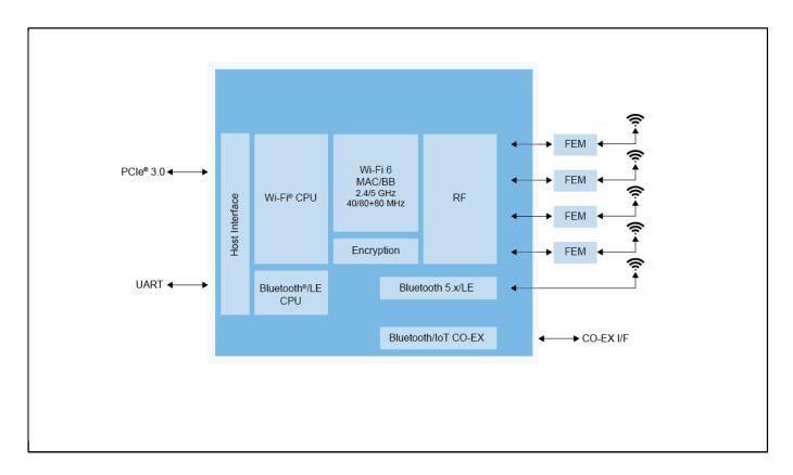
View additional information for 2.4/5 GHz Dual-Band 4x4 Wi-Fi® 6 (802.11ax) Access Solution.
