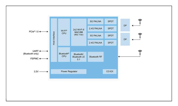
View additional information for 2.4/5 GHz Dual-Band 2x2 Wi-Fi® 6 (802.11ax) + Bluetooth® 5.1 Solution.
