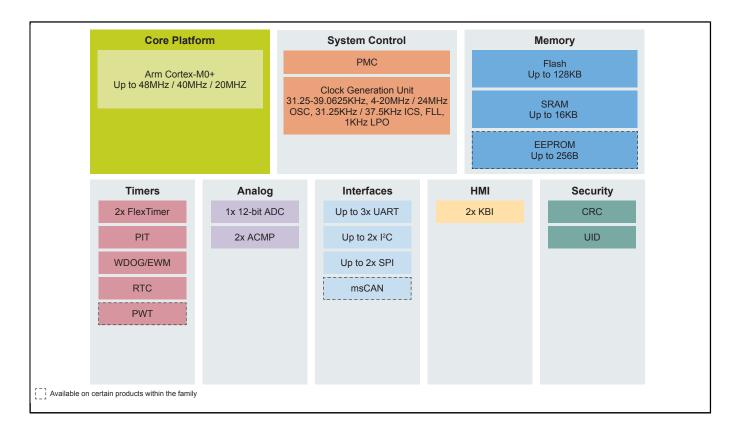
View additional information for Kinetis® KE06-48 MHz, Mainstream with CAN Microcontrollers (MCUs) based on Arm® Cortex®-M0+ Core.
