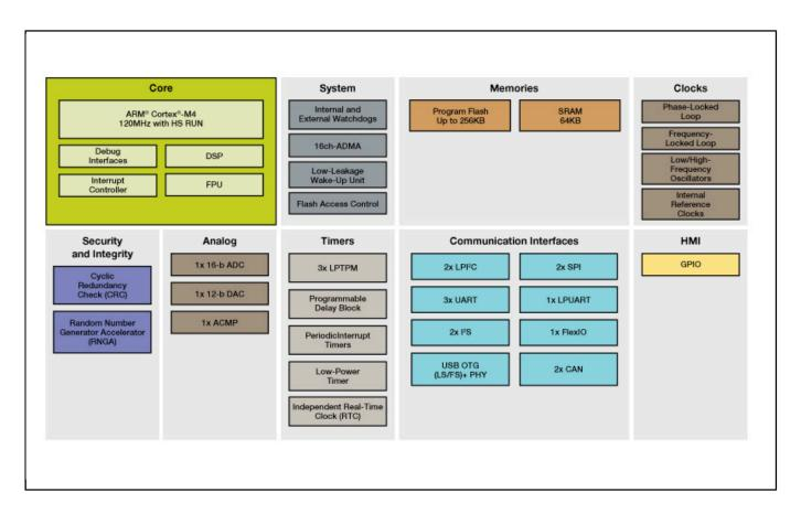
View additional information for KS22 and KS20 Arm® Cortex®-M4 Microcontrollers with USB and Dual CAN.
