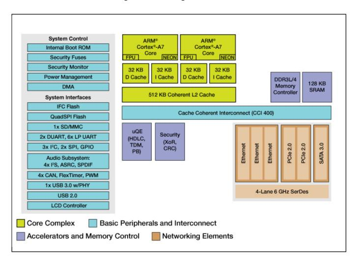
View additional information for Layerscape® 1021A Dual-Core Processor with LCD Controller.
