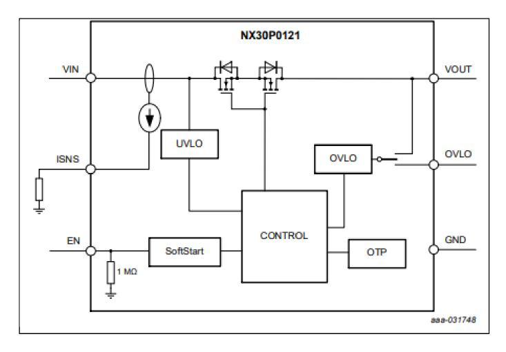
View additional information for High-Voltage Back-to-Back OVP Switch with Current Sense.
