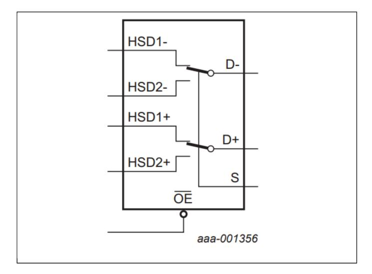
View additional information for Dual High-Speed USB 2.0 Double-Pole Double-Throw Analog Switch.
