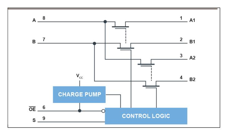
View additional information for I3C Switch with Hardware Select and Enable.
