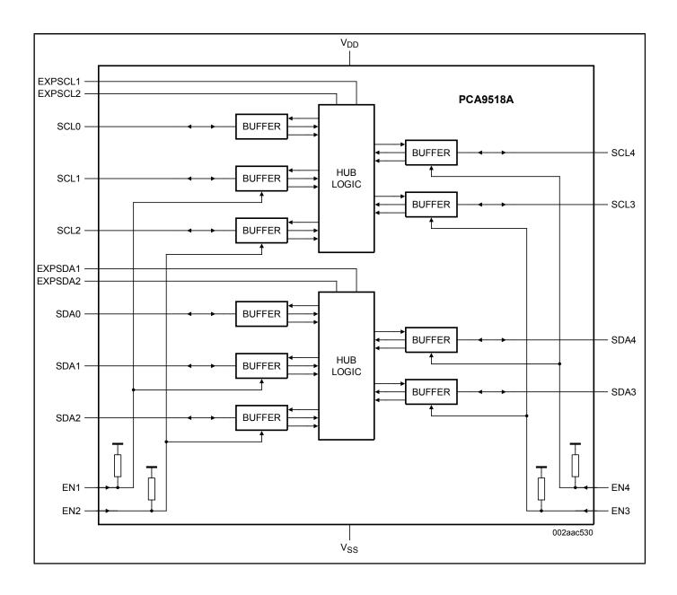
Block diagram: PCA9518AD, PCA9518APW Block Diagram
