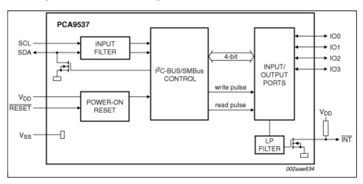
View additional information for 4-Bit I<sup>2</sup>C-Bus and SMBus Low-Power I/O Port with Interrupt and Reset.
