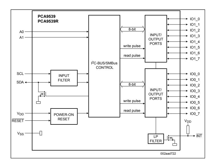
PCA9539BS, PCA9539D, PCA9539PW, PCA9539RBS, PCA9539RPW Block Diagram
