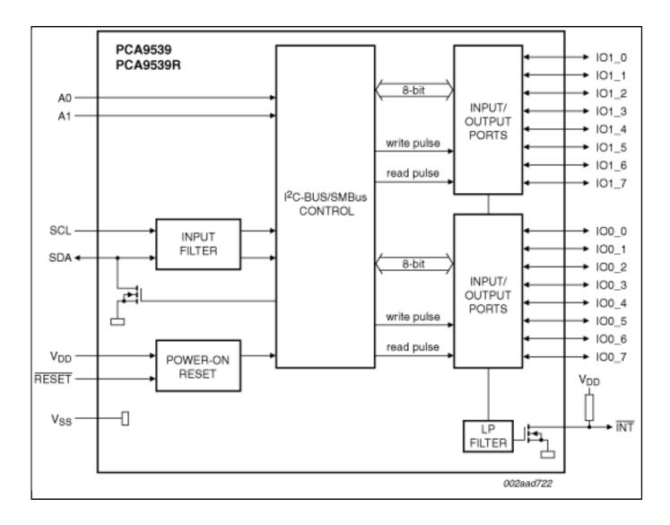
View additional information for 16-Bit I2C-Bus and SMBus Low-Power I/O Port with Interrupt and Reset.
