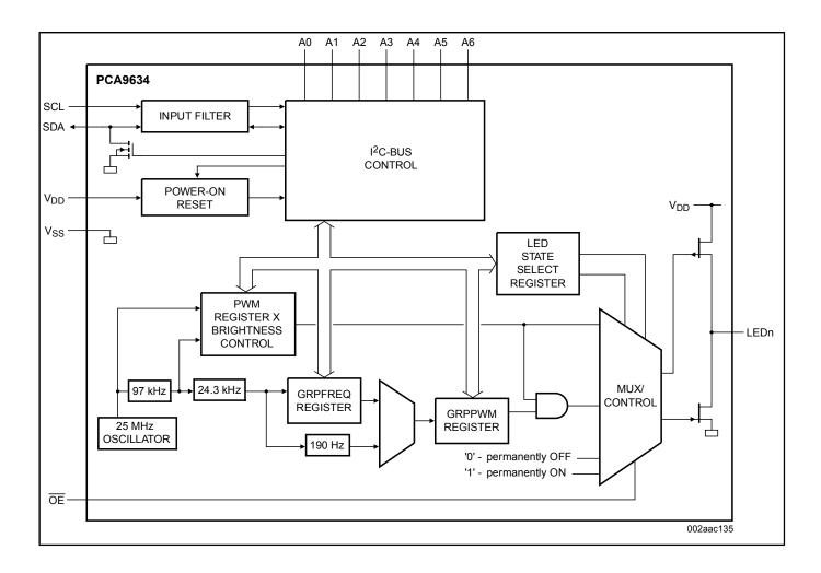
Block diagram: PCA9634BS, PCA9634D, PCA9634PW Block Diagram
