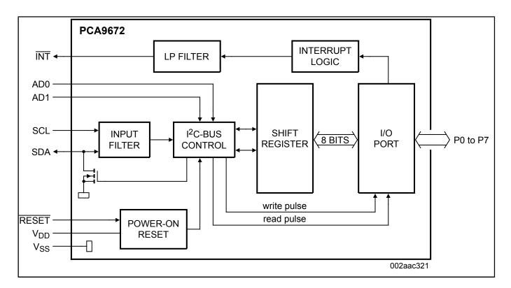
PCA9672BS, PCA9672D, PCA9672PW Block Diagram
