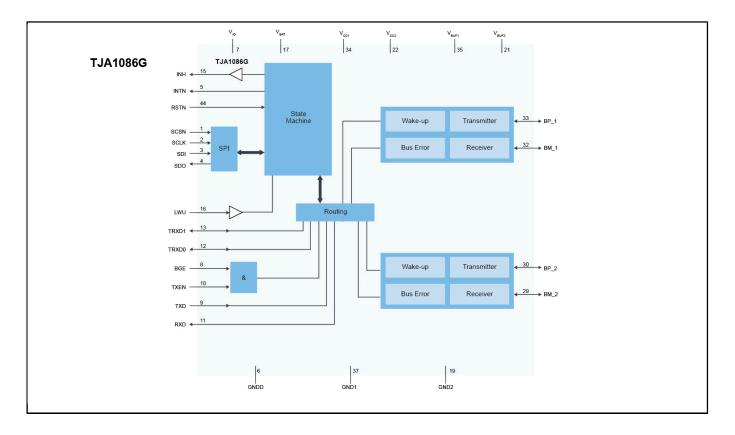
Active star coupler that connects two branches of a FlexRay network Block Diagram
