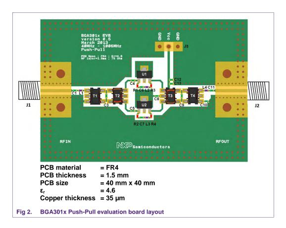
For optimum distortion performance it is important to have enough ground vias underneath and around the MMICs ground pins. This lowers the inductance to the ground plane. The evaluation board is made with two layer FR4 material.
