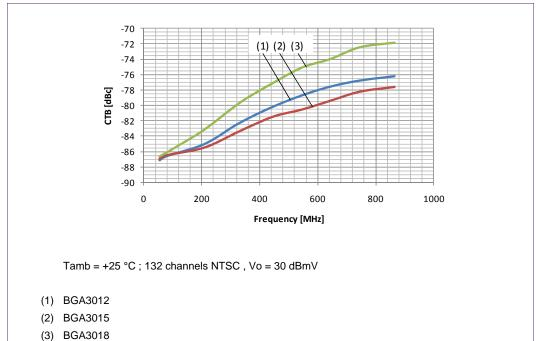
Fig 7. Composite triple beat (CTB); Vcc = 8 V
