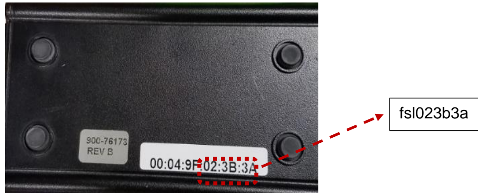
Figure 3: Last six digits of the MAC address as found on CWTAP label
