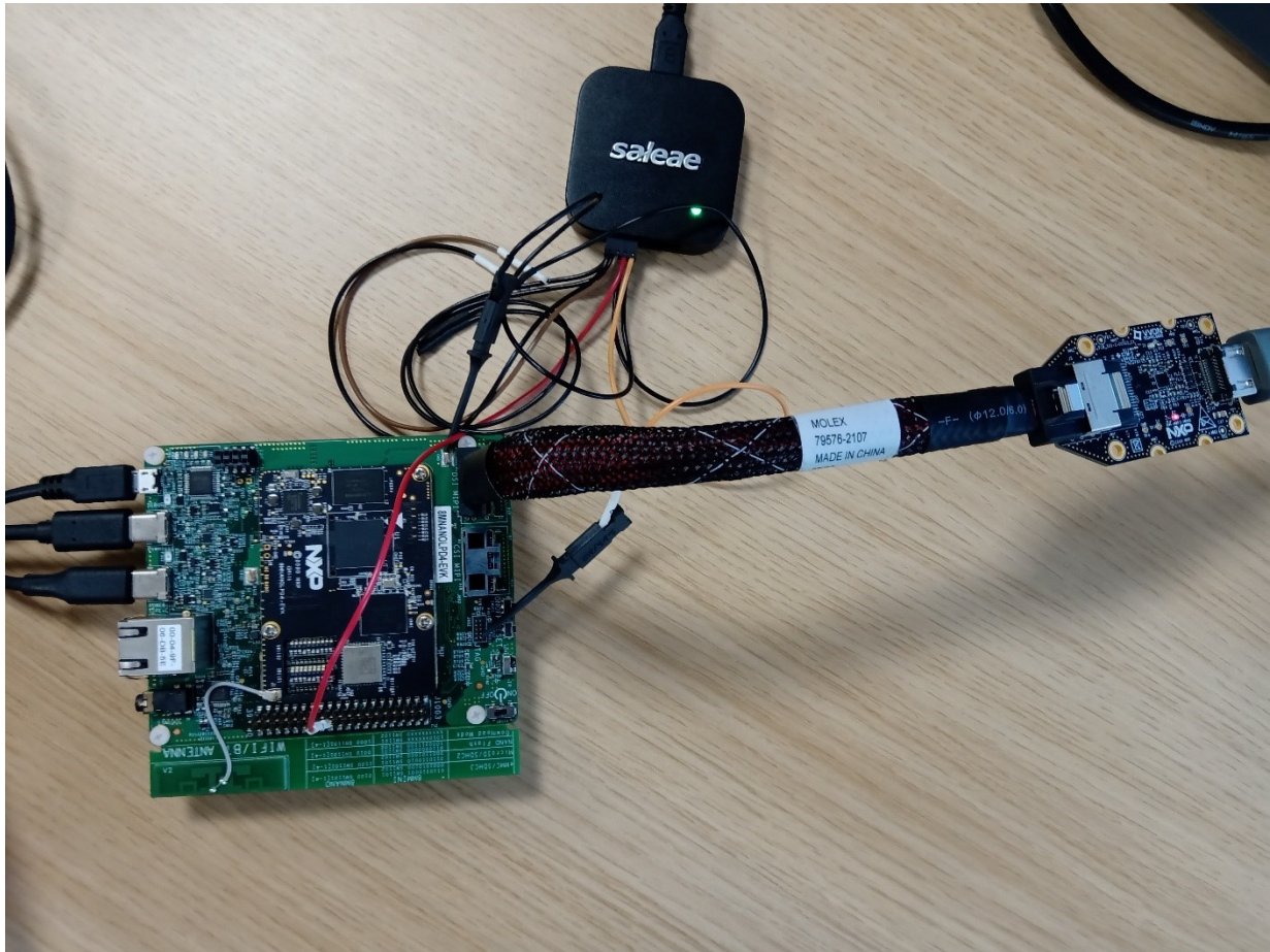
Figure 19. Measurement setup on the i.MX 8MN EVK board
