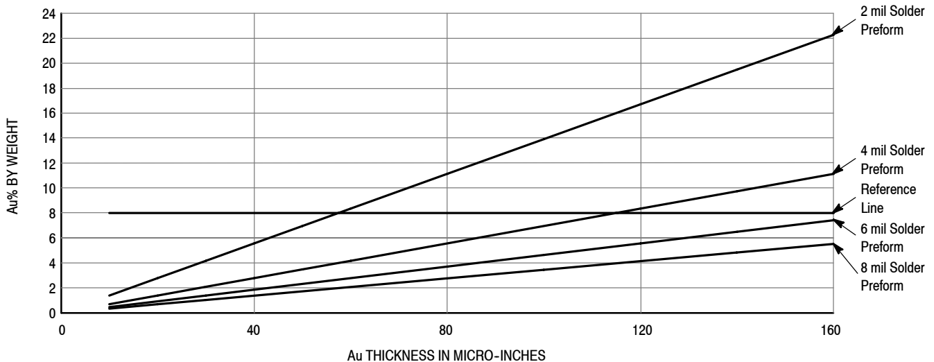
Figure 11. Percentage of Au in SnAgCu Solder for Various Thickness of Solder Preform
