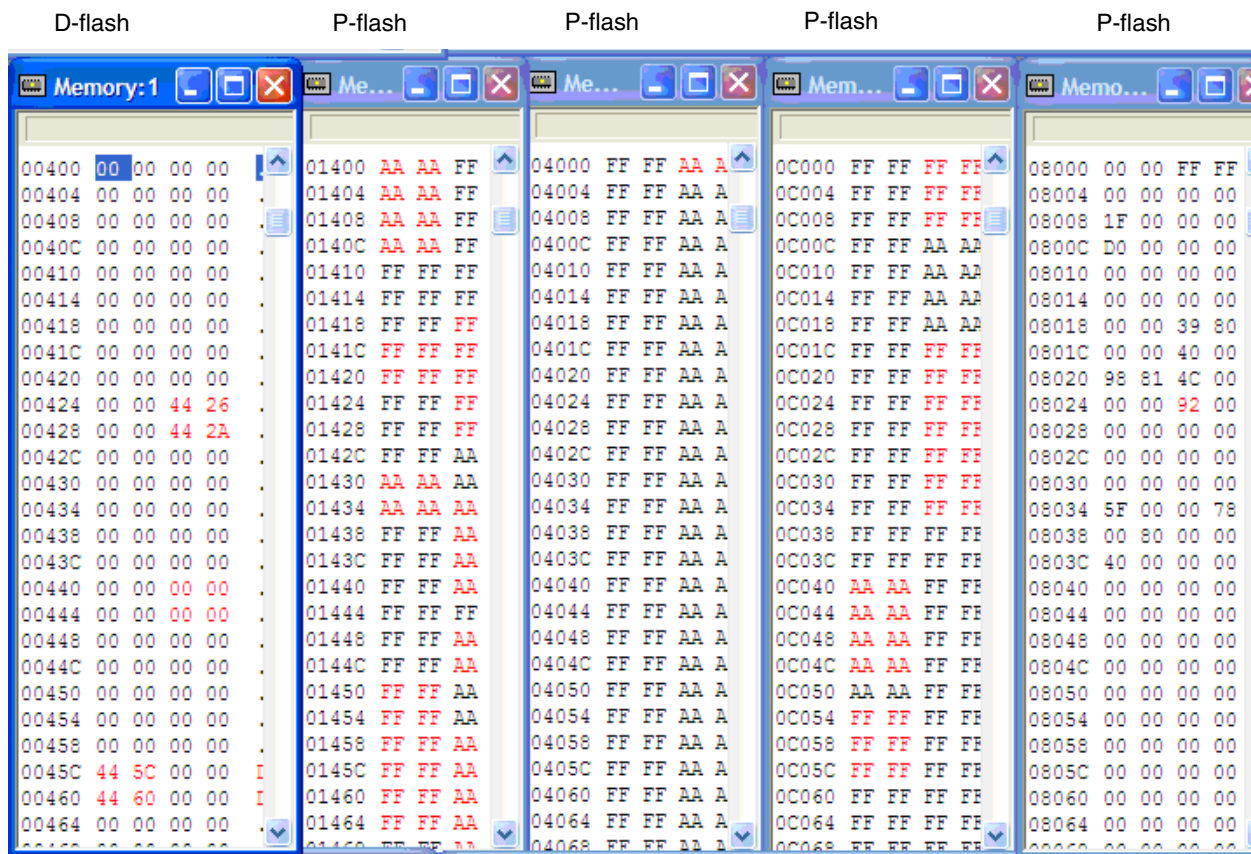
Figure 2. The memory maps showing real time erasing and programming
