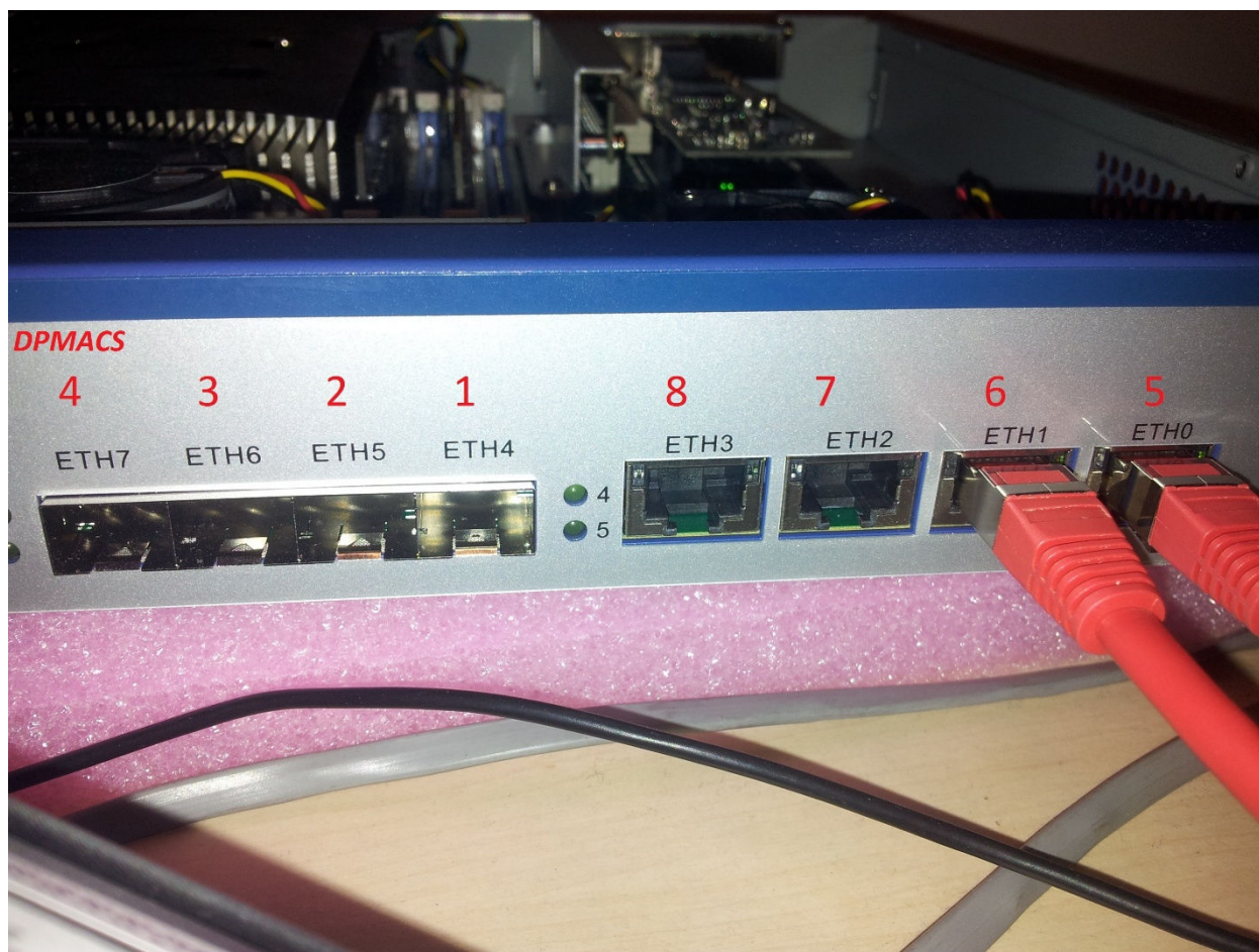
Figure 1. Hardware setup using one board with two ports connected back-to-back
