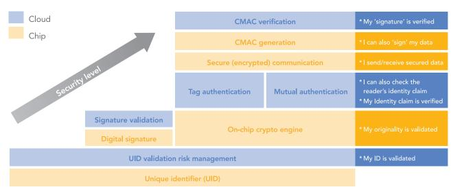
Our most advanced NXP DNA product line – NTAG® 424 DNA and NTAG 424 DNA TagTamper - includes AES-128 hardware for cryptographic operations on attack-resistant silicon. The DNA products use symmetric cryptography, with the same key for encryption and decryption, to safeguard information. The main advantage of symmetric algorithms is their efficiency and speed of execution, to manage digital signing and authentication applications.
