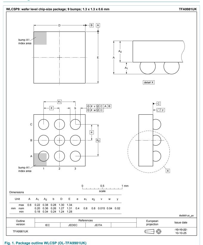
Wafer level chip-size package; 9 bumps; 1.3 x 1.3 x 0.6 mm
