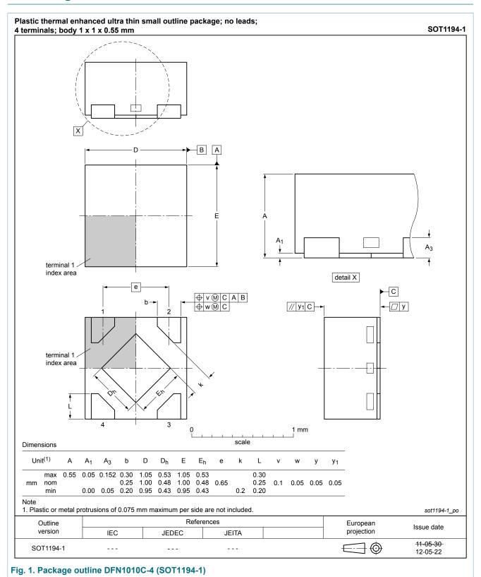
DFN1010C-4: plastic thermal enhanced ultra thin small outline package; no leads; 4 terminals
