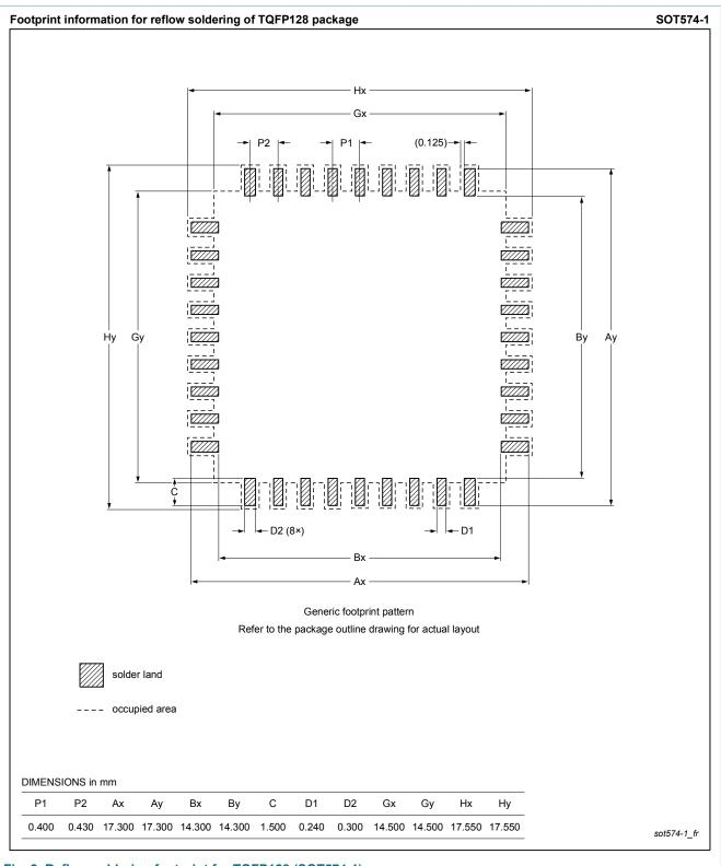
Fig. 2. Reflow soldering footprint for TQFP128 (SOT574-1)
