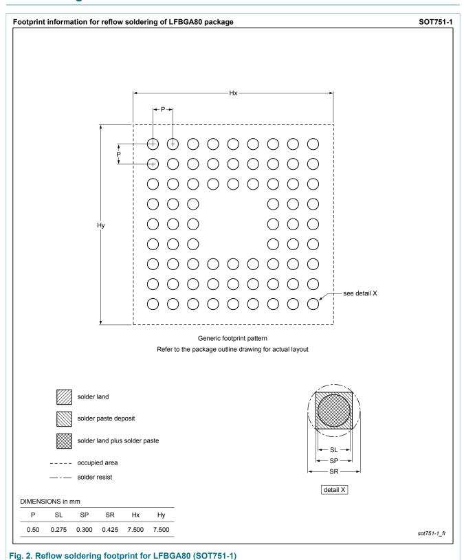
plastic low profile fine-pitch ball grid array package; 80 balls; body 7 x 7 x 1.05 mm
