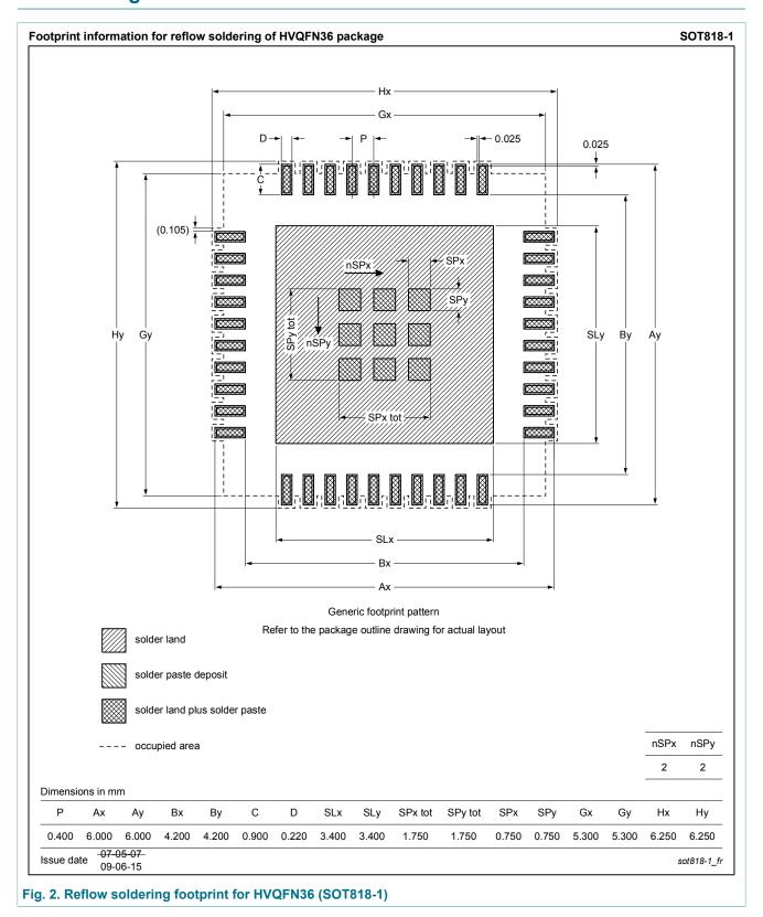
plastic thermal enhanced very thin quad flat package; no leads; 36 terminals; body 5 x 5 x 0.85 mm
