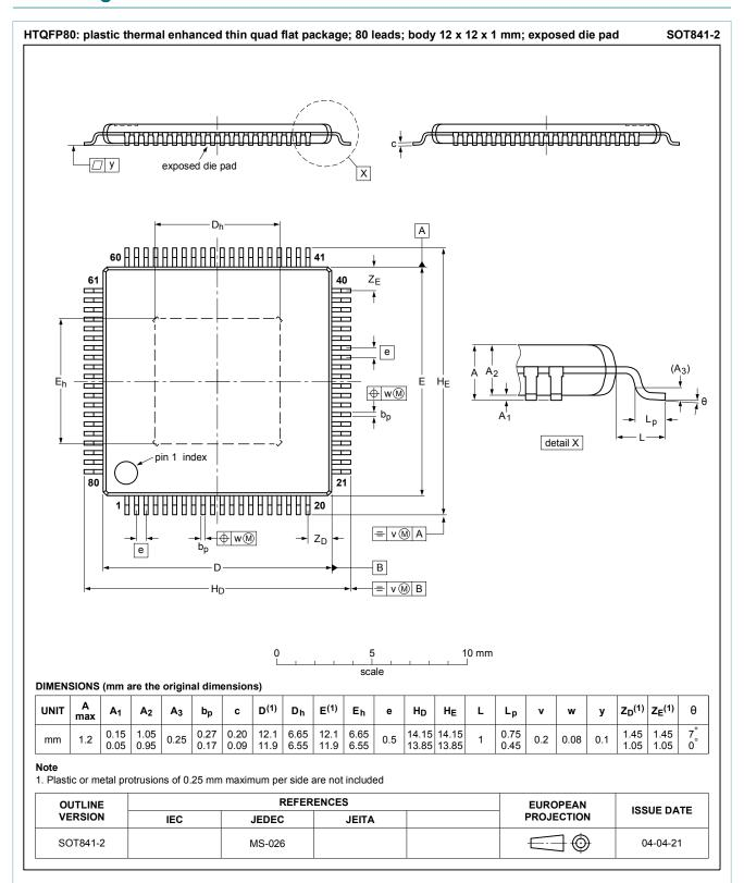
plastic thermal enhanced thin quad flat package; 80 leads; body 12 x 12 x 1 mm; exposed die pad
