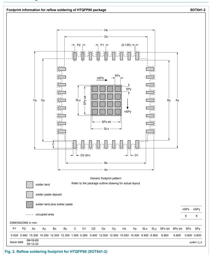
plastic thermal enhanced thin quad flat package; 80 leads; body 12 x 12 x 1 mm; exposed die pad
