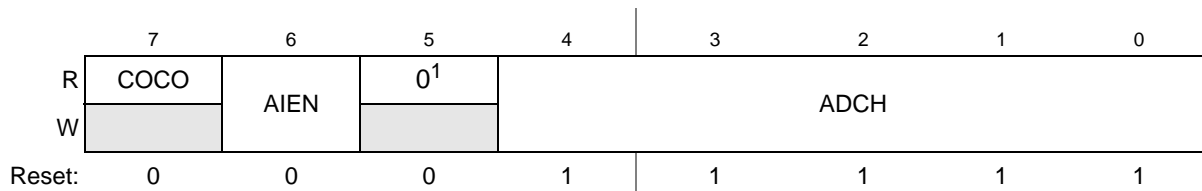
Figure 10-4. Status and Channel Control Register 1n (ADCSC1)
