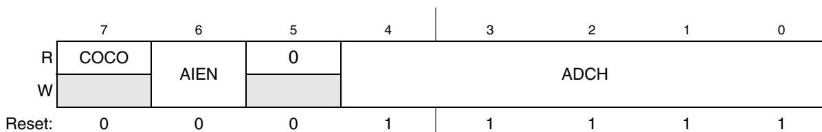
Figure 11-3. Status and Channel Control Register 1n (ADCSC1)
