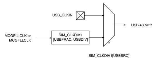
Figure 5-2. USB 48 MHz Clock Source
