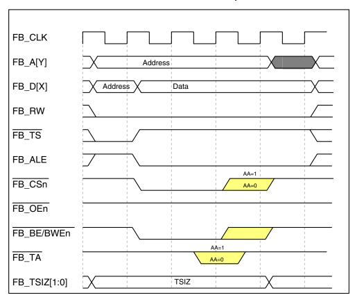
Figure 25-24. Write-Bus Cycle (One Wait State)
