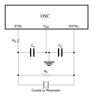
Figure 22-5. Crystal/Ceramic Resonator Connections - Connection 4
