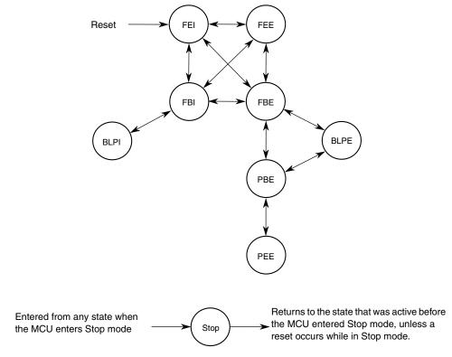
Figure 21-12. MCG mode state diagram
