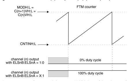
Figure 38-171. Channel (n) output if (C(n)V = C(n+1)V = MOD)
