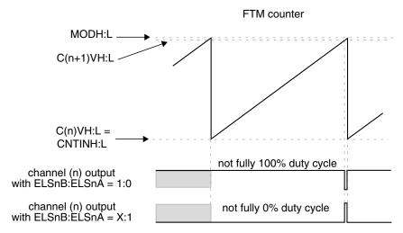
Figure 38-167. Channel (n) output if (C(n)V = CNTIN) and (CNTIN < C(n+1)V < MOD) and (C(n+1)V) is almost equal to (C(n+1)V)
