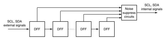
Figure 43-65. Programmable input glitch filter diagram
