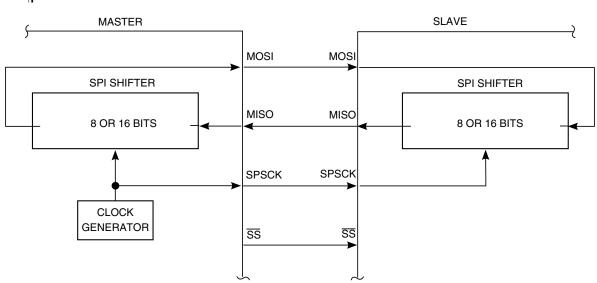
Figure 39-1. SPI System Connections
