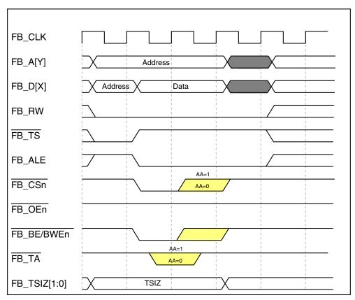
Figure 25-22. Basic Write-Bus Cycle (No Wait States)
