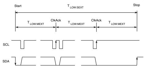
Figure 43-64. Timeout measurement intervals
