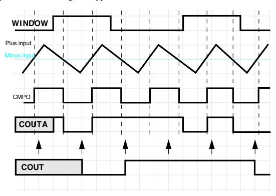
Figure 31-22. Windowed/resampled mode operation
