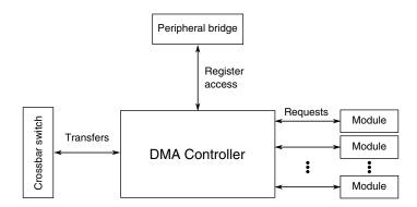
Figure 3-5. DMA Controller configuration
