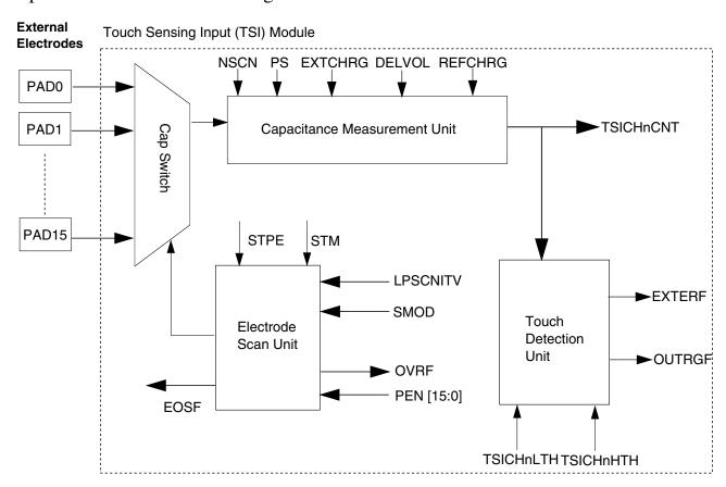
Figure 49-1. Touch sensing input block diagram
