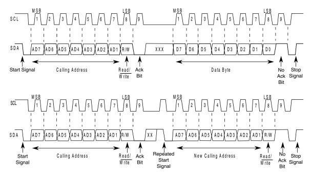
Figure 43-62. I2C bus transmission signals
