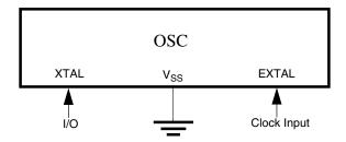
Figure 22-6. External Clock Connections
