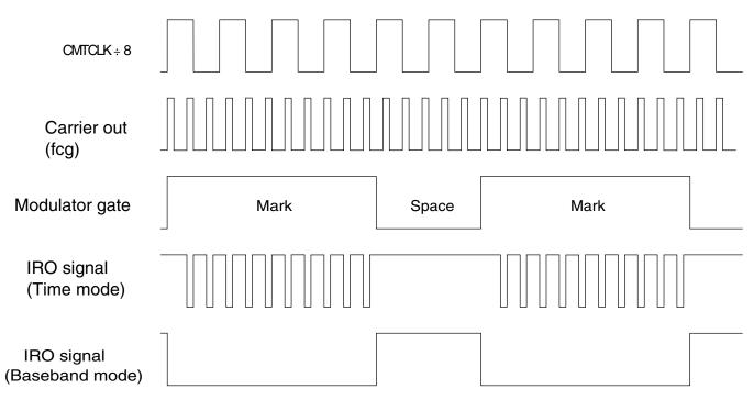
Figure 37-17. Example: CMT output in Time and Baseband modes with OC[CMTPOL]=0
