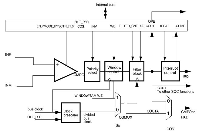
Figure 31-2. Comparator module block diagram
