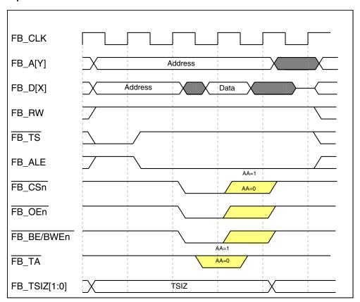
Figure 25-25. Read-Bus Cycle with Two-Clock Address Setup (No Wait States)
