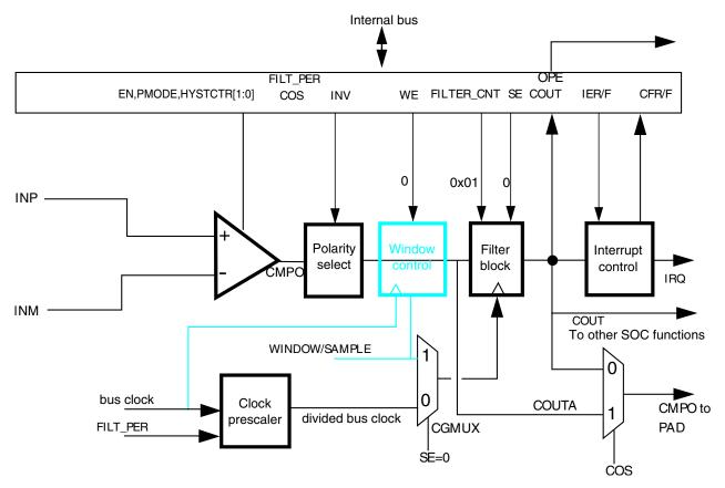
Figure 31-17. Sampled, Non-Filtered (# 3B): sampling interval internally derived
