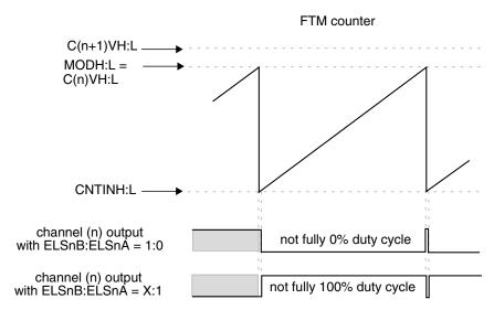
Figure 38-177. Channel (n) output if (C(n+1)V > MOD) and (CNTIN < C(n)V = MOD)
