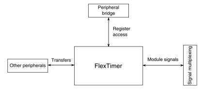
Figure 3-30. FlexTimer configuration
