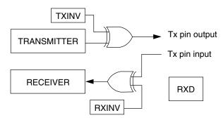
Figure 44-114. Single-wire operation (C1[LOOPS] = 1, C1[RSRC] = 1)
