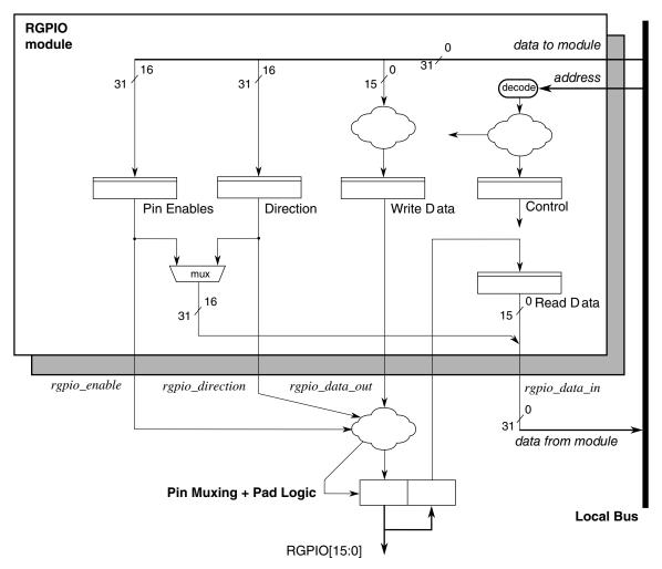
Figure 46-1. RGPIO Block Diagram
