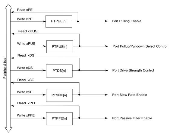
Figure 47-80. Diagram of PCTRL function
