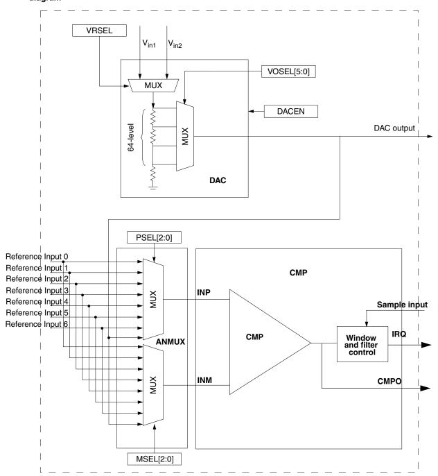
Figure 31-1. CMP, DAC and ANMUX block diagram
