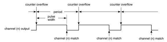
Figure 38-156. EPWM period and pulse width with ELSnB:ELSnA = 1:0
