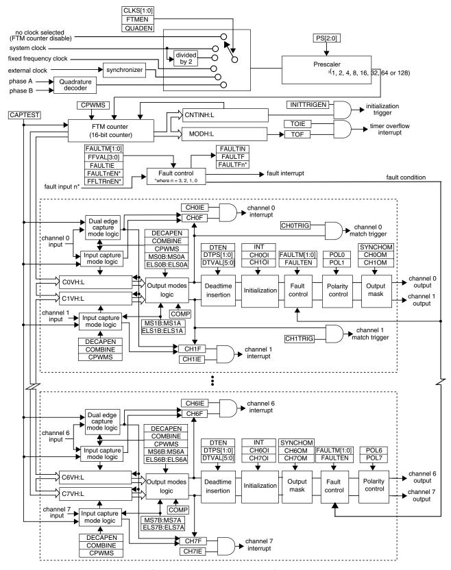
Figure 38-1. FTM block diagram
