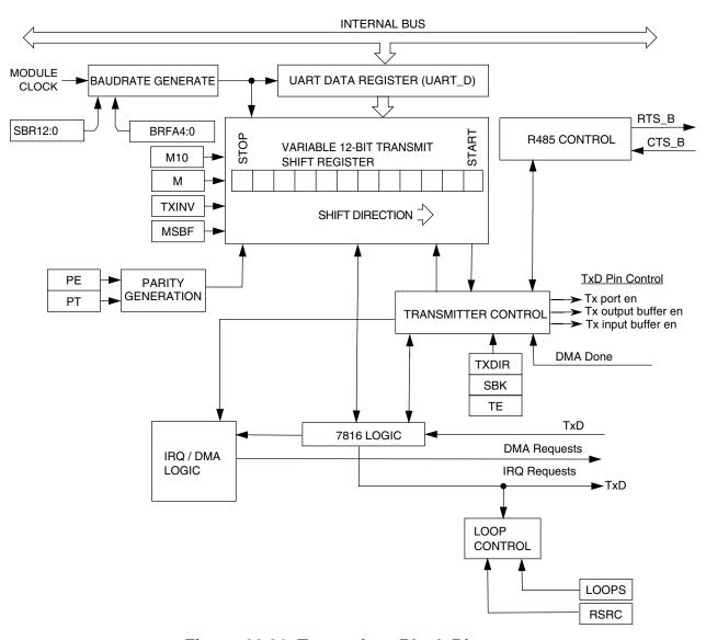
Figure 44-91. Transmitter Block Diagram
