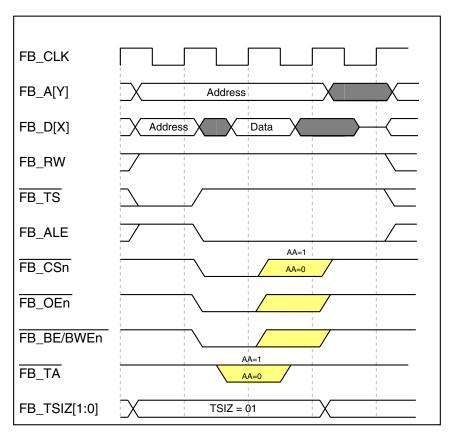
Figure 25-17. Single Byte-Read Transfer
