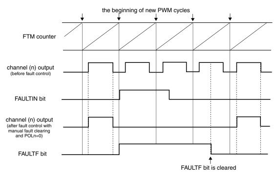
Figure 38-202. Fault control with manual fault clearing
