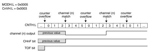
Figure 38-153. Example of the output compare mode when the match toggles the channel output
