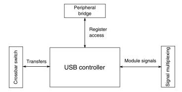
Figure 3-38. USB controller configuration
