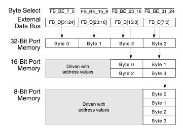
Figure 25-12. Connections for external memory port sizes (CSCRn[BLS] = 1)
