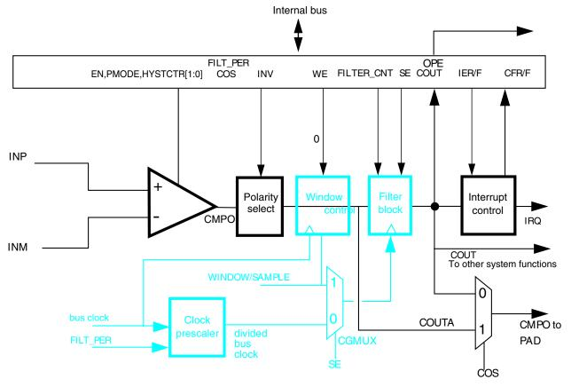
Figure 31-15. Comparator operation in Continuous mode
