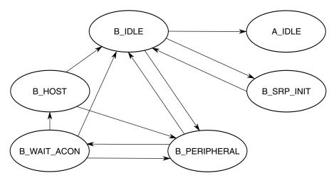
Figure 40-94. Dual role B device flow diagram
