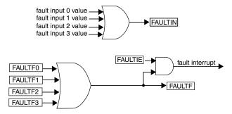
Figure 38-200. FAULTF and FAULTIN bits and fault interrupt
