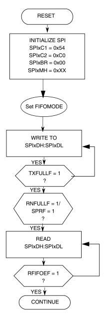
Figure 39-42. Initialization Flowchart Example for SPI Master Device in 16-bit Mode for FIFOMODE = 1
