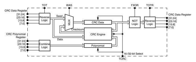
Figure 29-1. Programmable cyclic redundancy check (CRC) block diagram
