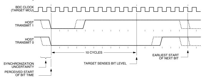
Figure 51-3. BDC Host-to-Target Serial Bit Timing
