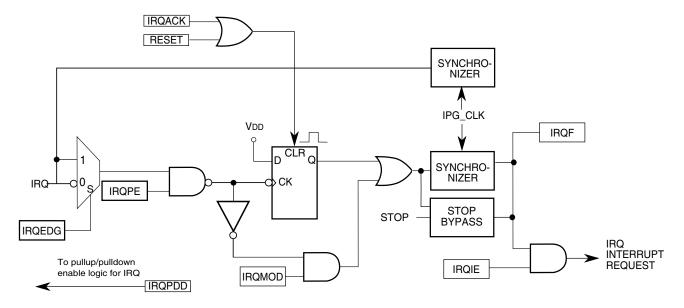
Figure 50-1. IRQ Block Diagram
