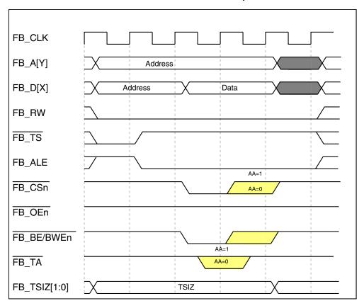
Figure 25-26. Write-Bus Cycle with Two Clock Address Setup (No Wait States)
