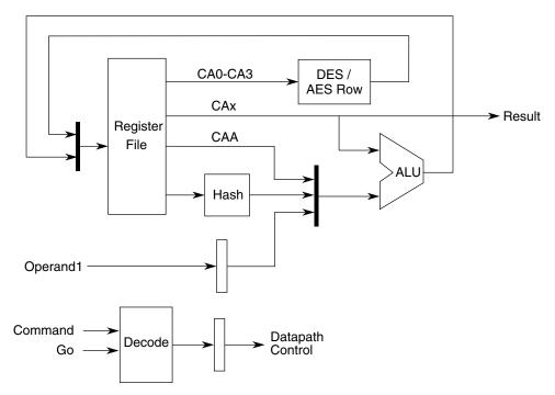
Figure 27-1. Top-level CAU block diagram
