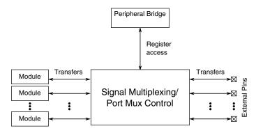
Figure 9-1. Signal multiplexing integration
