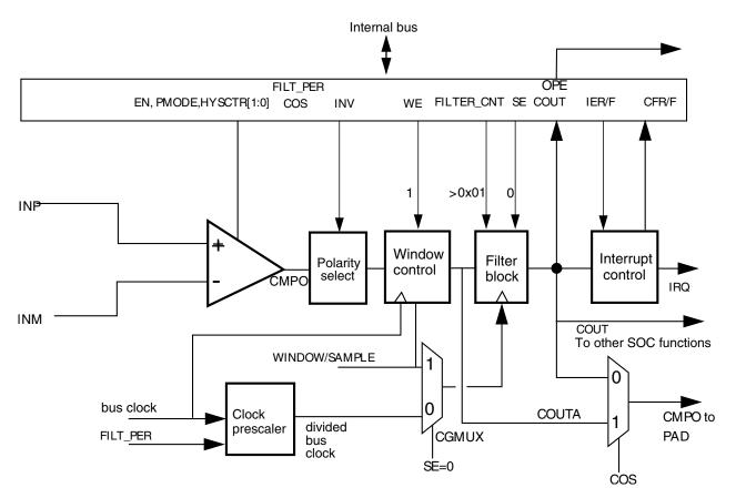
Figure 31-23. Windowed/Filtered mode
