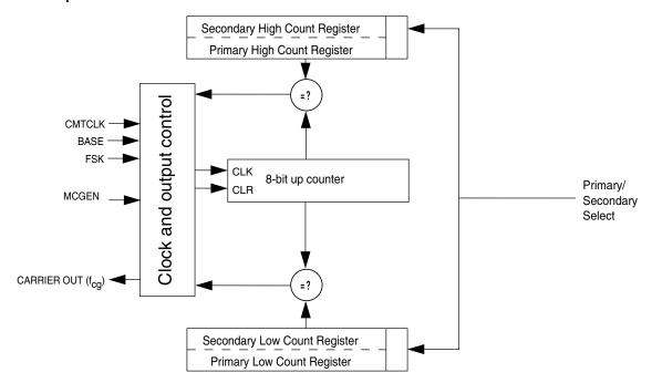
Figure 37-15. Carrier generator block diagram
