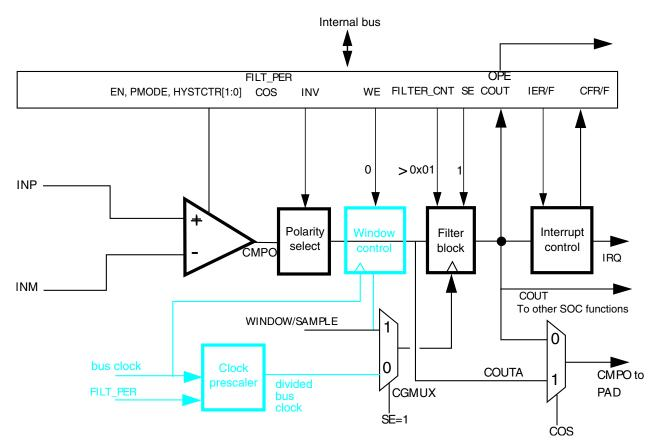
Figure 31-18. Sampled, Filtered (# 4A): sampling point externally driven
