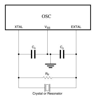
Figure 22-4. Crystal/Ceramic Resonator Connections - Connection 3
