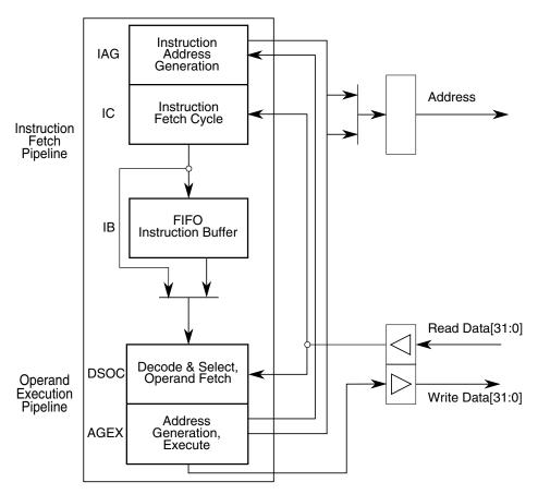
Figure 11-1. V1 ColdFire Core Pipelines
