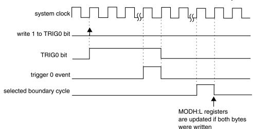
Figure 38-183. MODH:L synchronization when (PWMSYNC = 0), (REINIT = 0), and a hardware trigger was used
