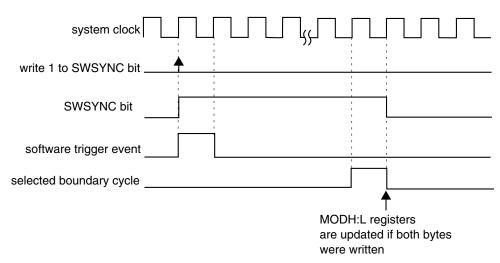
Figure 38-186. MODH:L synchronization when (PWMSYNC = 1)
