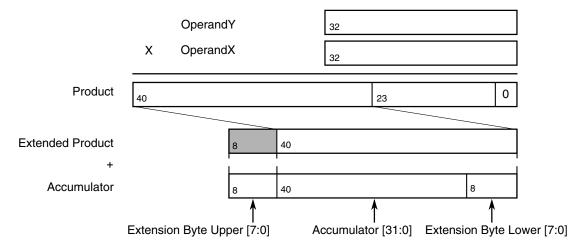
Figure 12-2. Fractional Alignment
