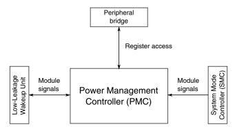
Figure 3-9. PMC configuration
