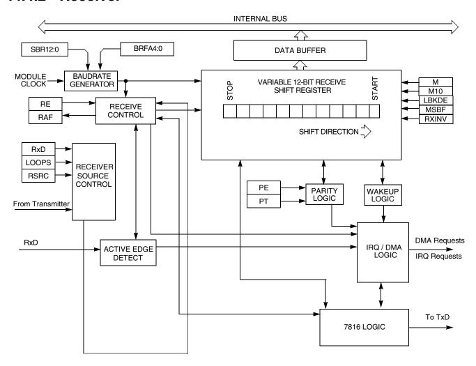
Figure 44-93. UART receiver block diagram
