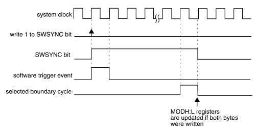
Figure 38-182. MODH:L synchronization when (PWMSYNC = 0), (REINIT = 0), and software trigger was used
