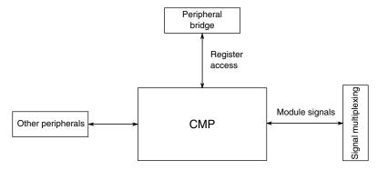
Figure 3-26. CMP configuration
