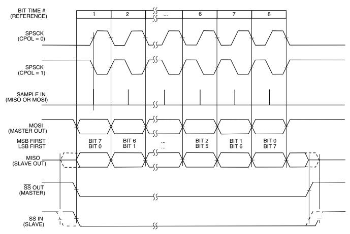
Figure 39-39. SPI Clock Formats (CPHA = 0)
