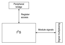
Figure 3-44. I<sup>2</sup>S configuration
