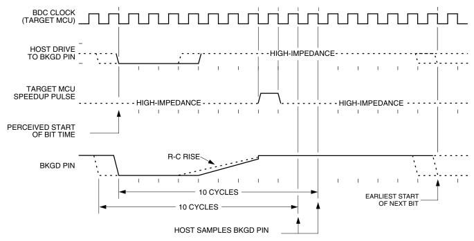
Figure 51-4. BDC Target-to-Host Serial Bit Timing (Logic 1)
