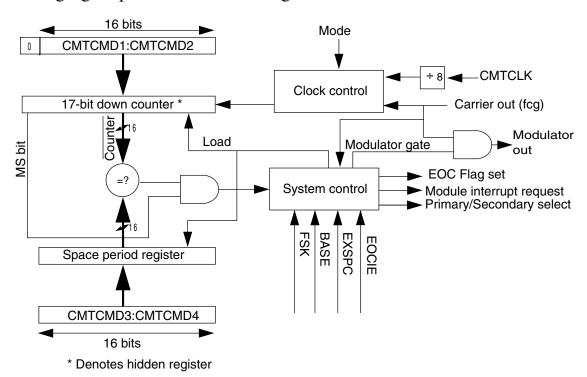
Figure 37-16. Modulator block diagram
