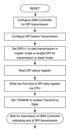
Figure 39-37. Recommended startup of SPI transmit by DMA
