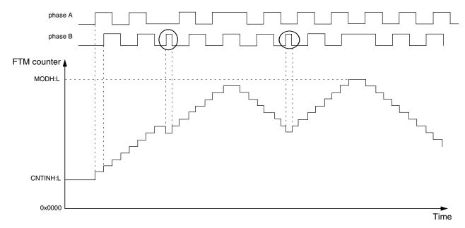
Figure 38-221. Motor Position Jittering in a Mid Count Value
