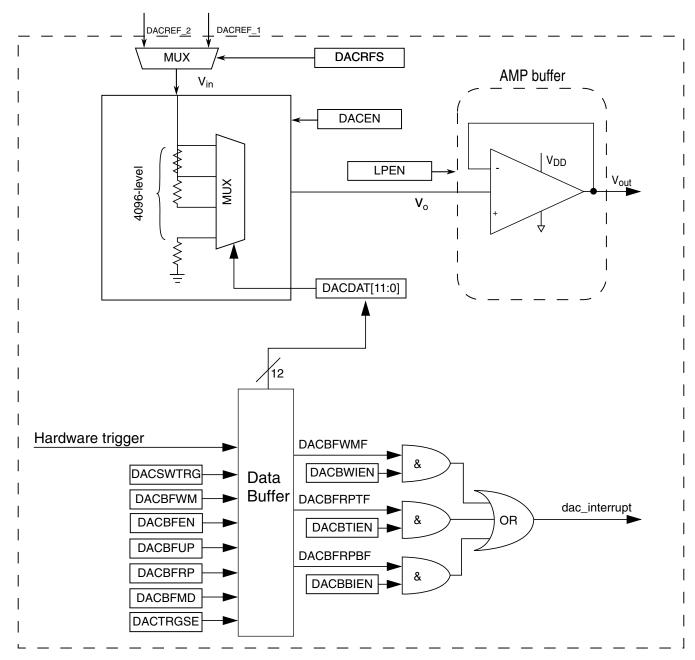
Figure 32-1. DAC block diagram
