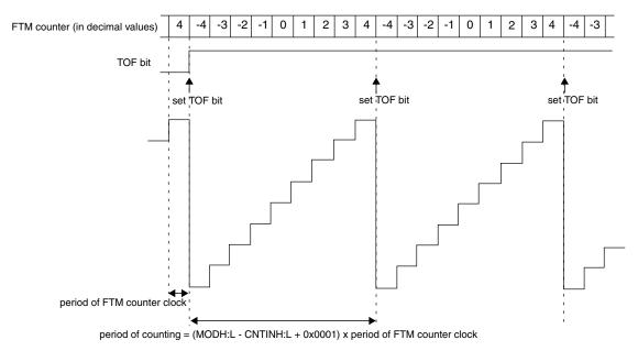
Figure 38-145. Example of FTM up and signed counting
