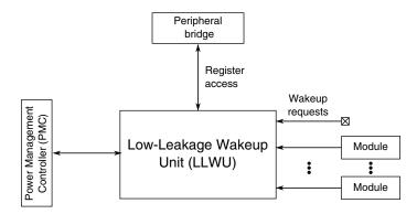
Figure 3-7. Low-Leakage Wakeup Unit configuration
