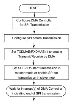
Figure 39-36. Basic Flow of SPI Transmission by DMA
