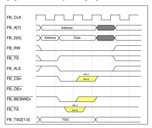
Figure 25-16. Basic Write-Bus Cycle
