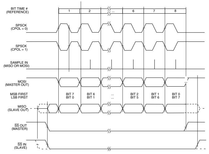
Figure 39-38. SPI Clock Formats (CPHA = 1)
