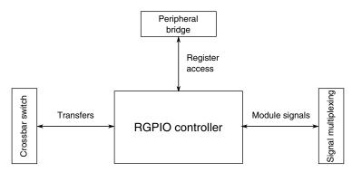
Figure 3-45. RGPIO configuration
