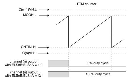
Figure 38-168. Channel (n) output if C(n)V and C(n+1)V are not between CNTIN and MOD
