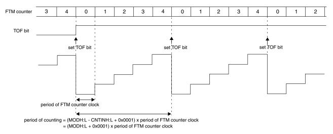
Figure 38-146. Example of FTM up counting with CNTIN = 0x0000
