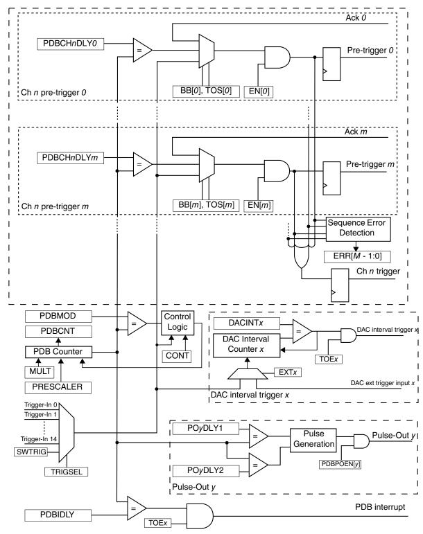
Figure 34-1. PDB block diagram
