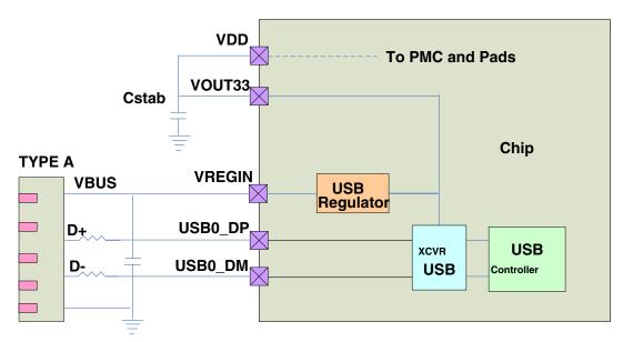
Figure 3-37. USB regulator bus supply
