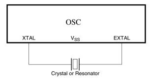
Figure 22-2. Crystal/Ceramic Resonator Connections - Connection 1
