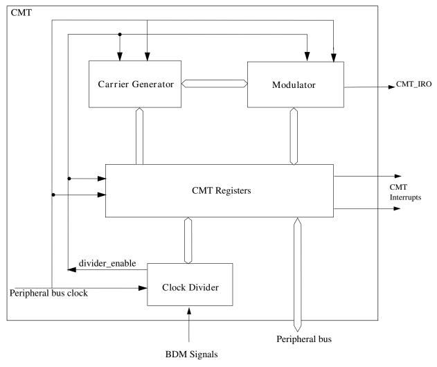
Figure 37-1. CMT module block diagram
