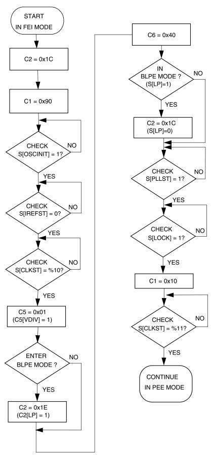
Figure 21-13. Flowchart of FEI to PEE mode transition using an 4 MHz crystal MCF51JF128 Reference Manual, Rev. 5, 08/2012
