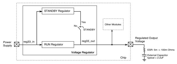
Figure 42-2. USB Voltage Regulator Block Diagram
