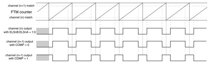
Figure 38-178. Channel (n+1) output in complementary mode with (ELSnB:ELSnA = 1:0)
