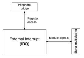
Figure 3-48. IRQ module configuration
