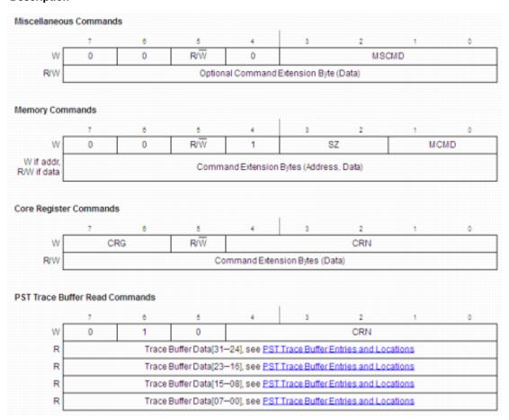
Figure 51-6. BDM Command Encodings
