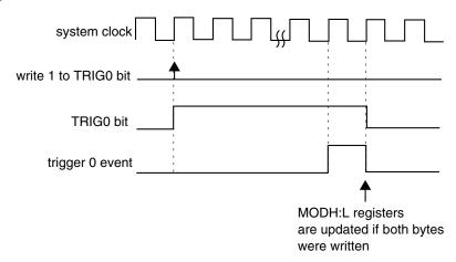
Figure 38-185. MODH:L synchronization when (PWMSYNC = 0), (REINIT = 1), and a hardware trigger was used
