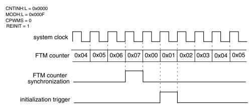
Figure 38-207. Initialization trigger is generated when there is the FTM counter synchronization
