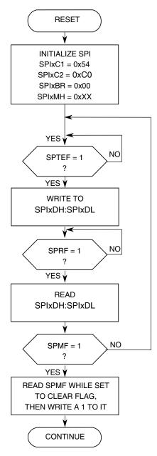
Figure 39-41. Initialization Flowchart Example for SPI Master Device in 16-bit Mode for FIFOMODE = 0
