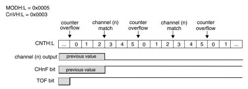
Figure 38-154. Example of the output compare mode when the match clears the channel output
