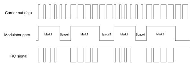
Figure 37-18. Example: CMT output in FSK mode
