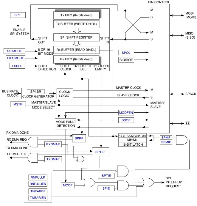
Figure 39-3. SPI Module Block Diagram with FIFO
