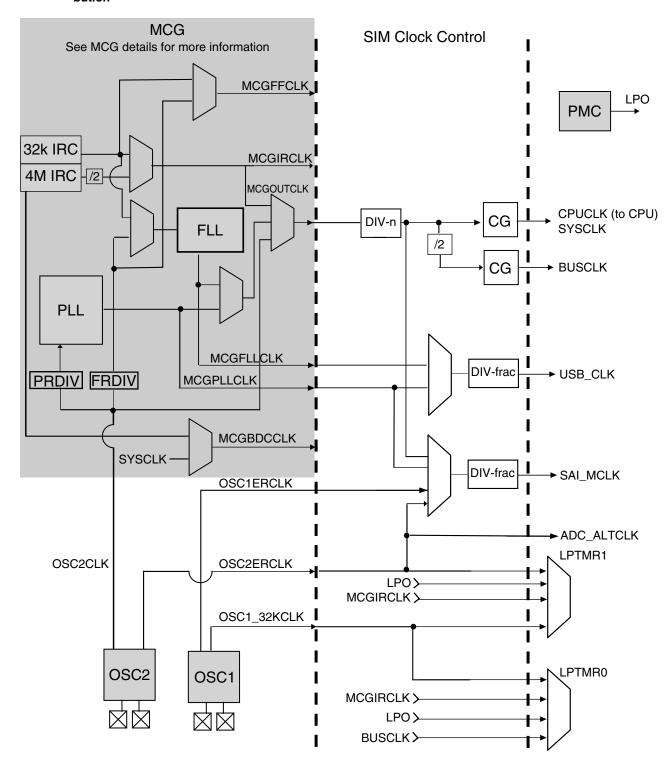
Figure 5-1. Clocking diagram
