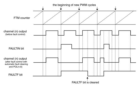
Figure 38-201. Fault control with automatic fault clearing
