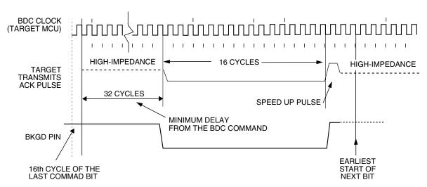
Figure 51-7. Target Acknowledge Pulse (ACK)
