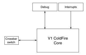
Figure 3-1. Core configuration
