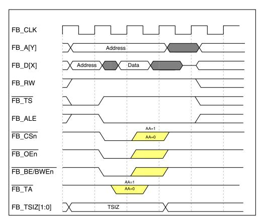
Figure 25-14. Basic Read-Bus Cycle
