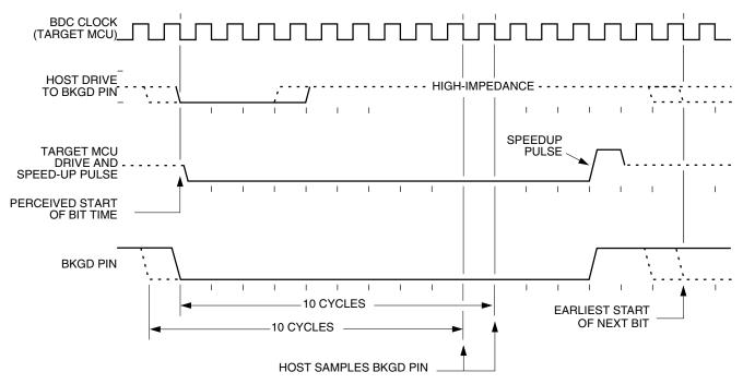
Figure 51-5. BDM Target-to-Host Serial Bit Timing (Logic 0)
