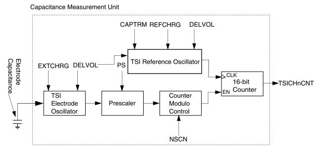
Figure 49-2. TSI capacitance measurement unit block diagram
