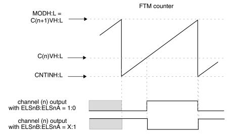
Figure 38-164. Channel (n) output if (CNTIN < C(n)V < MOD) and (C(n+1)V = MOD)
