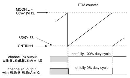
Figure 38-166. Channel (n) output if (CNTIN < C(n)V < MOD) and (C(n)V is almost equal to CNTIN) and (C(n+1)V = MOD)
