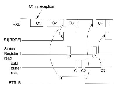
Figure 44-101. Receiver hardware flow control timing diagram
