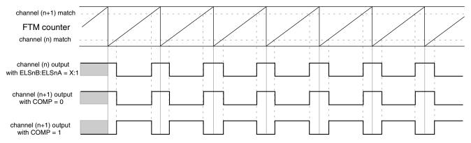
Figure 38-179. Channel (n+1) output in complementary mode with (ELSnB:ELSnA = X:1)
