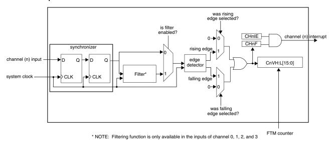
Figure 38-150. Input capture mode
