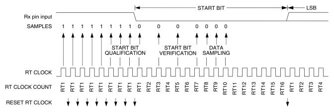
Figure 44-94. Receiver data sampling
