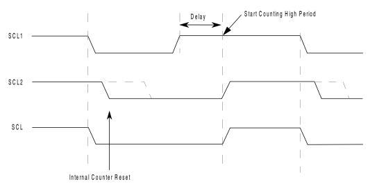
Figure 43-63. I2C clock synchronization
