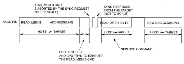
Figure 51-9. ACK Abort Procedure at the Command Level
