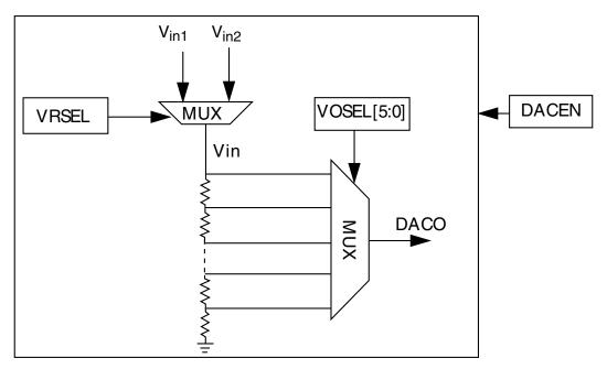
Figure 31-24. 6-bit DAC block diagram
