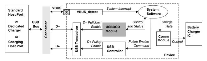
Figure 41-8. USB battery charging subsystem
