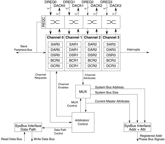
Figure 20-1. 4-Channel DMA Block Diagram
