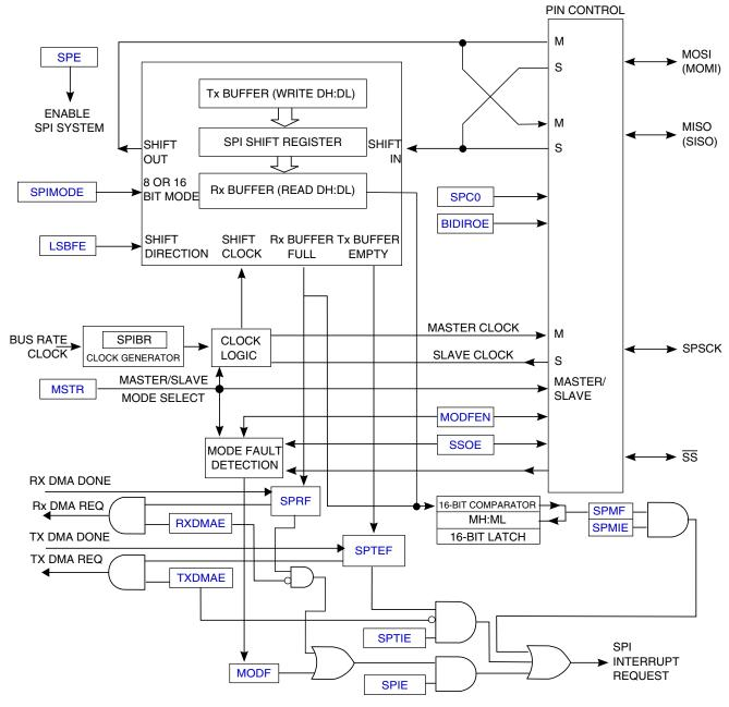
Figure 39-2. SPI Module Block Diagram without FIFO
