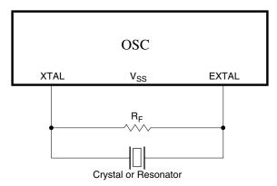
Figure 22-3. Crystal/Ceramic Resonator Connections - Connection 2
