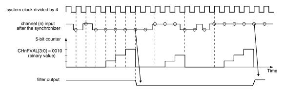
Figure 38-152. Channel input filter example
