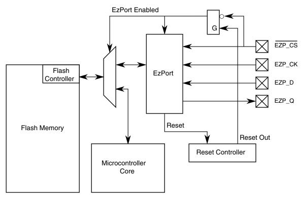
Figure 26-1. EzPort block diagram
