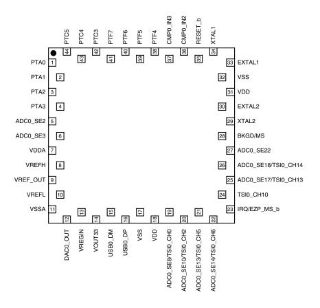
Figure 9-4. 44-pin Laminate QFN
