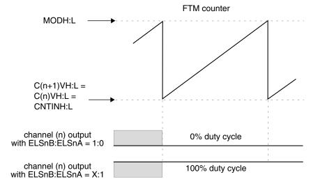
Figure 38-170. Channel (n) output if (C(n)V = C(n+1)V = CNTIN)
