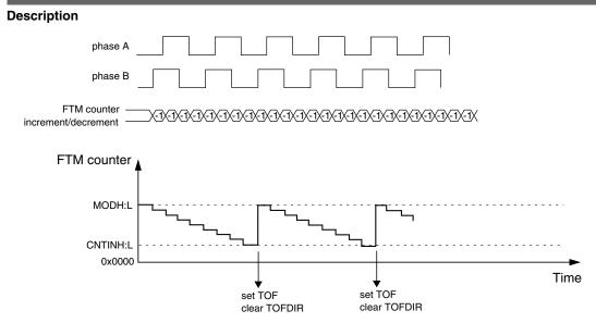
Figure 38-220. FTM Counter Overflow in Down Counting for Quadrature Decoder Mode
