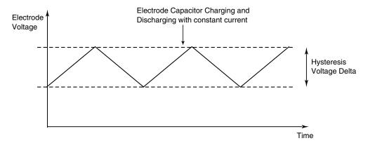
Figure 49-65. TSI electrode oscillator chart
