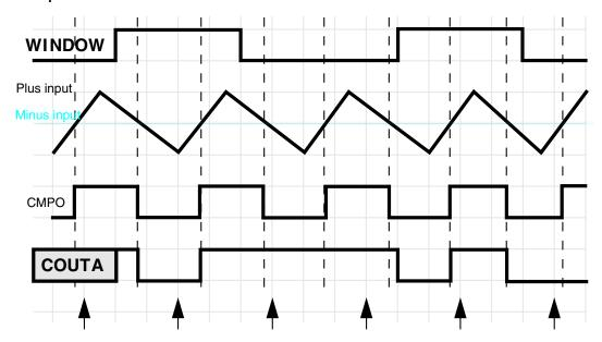
Figure 31-20. Windowed mode operation
