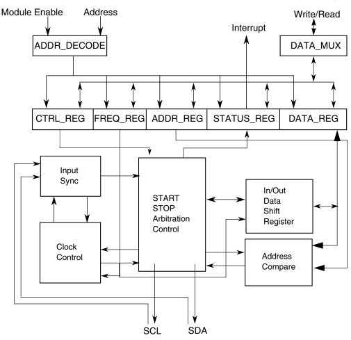
Figure 43-1. I2C Functional block diagram
