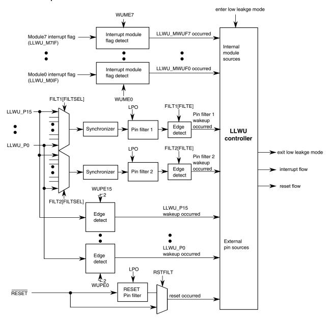
Figure 16-1. LLWU block diagram
