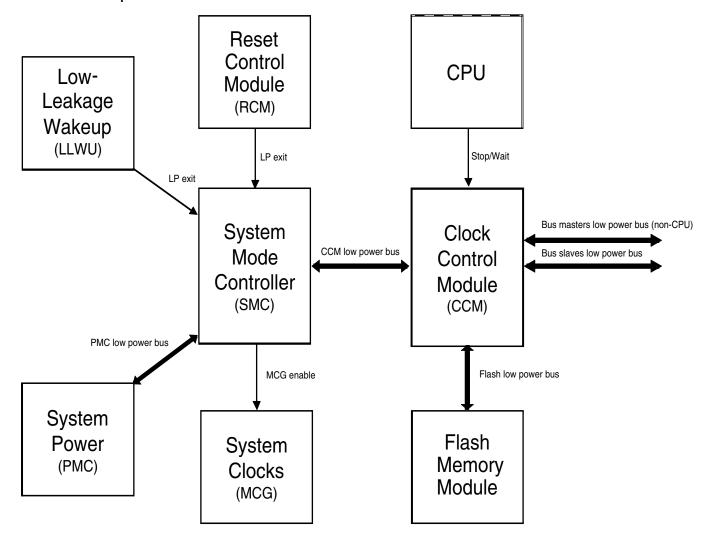
Figure 18-6. Low-power system components and connections
