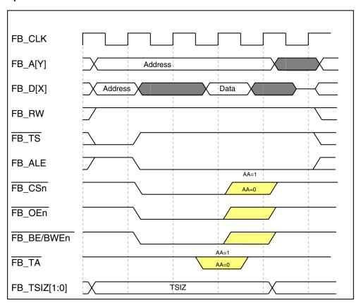
Figure 25-23. Read-Bus Cycle (One Wait State)
