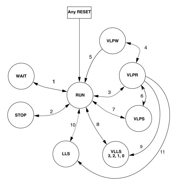
Figure 18-5. Power mode state diagram
