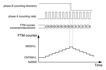
Figure 38-217. Quadrature Decoder – Count and Direction Encoding Mode
