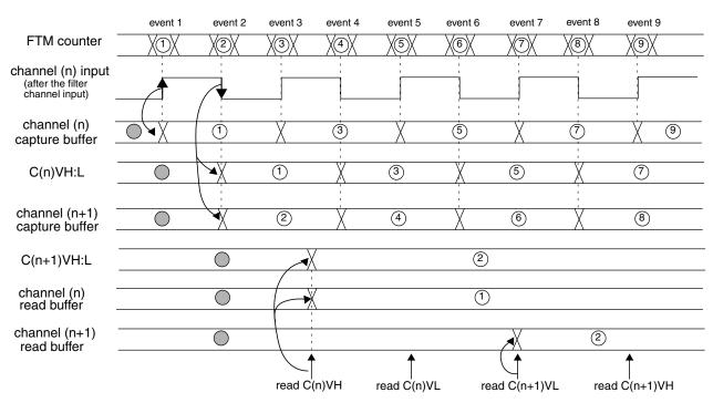
Figure 38-215. Dual edge capture mode read coherency mechanism
