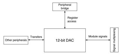
Figure 3-27. 12-bit DAC configuration
