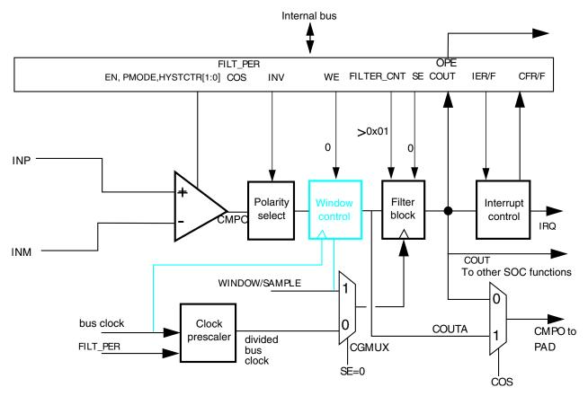
Figure 31-19. Sampled, Filtered (# 4B): sampling point internally derived
