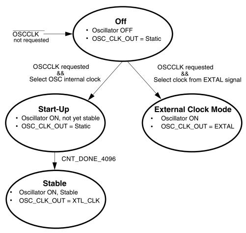
Figure 22-13. OSC Module State Diagram
