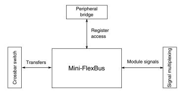
Figure 3-21. Mini-FlexBus configuration
