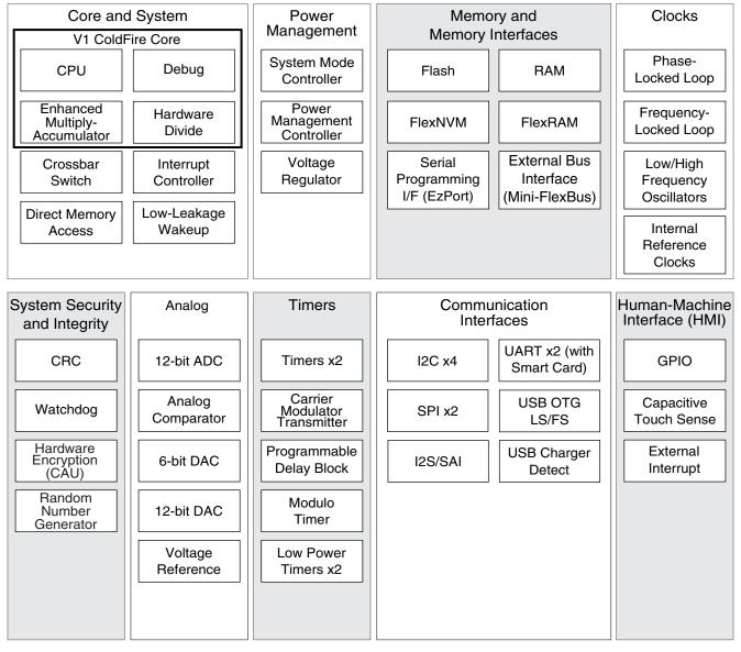
Figure 2-2. MCF51JF128 (64-pin) Block Diagram
