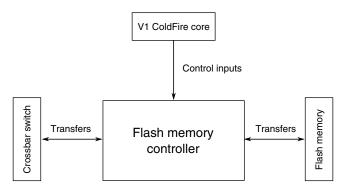
Figure 3-16. Flash memory controller configuration
