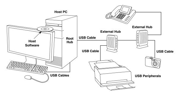
Figure 40-1. Example USB 2.0 system configuration
