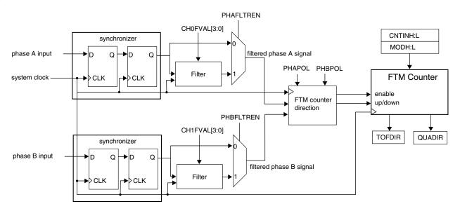
Figure 38-216. Quadrature Decoder Block Diagram
