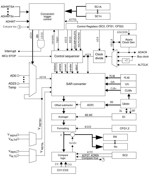
Figure 30-1. ADC block diagram
