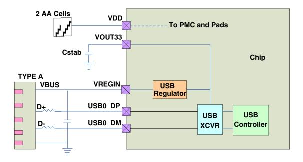
Figure 3-35. USB regulator AA cell use case
