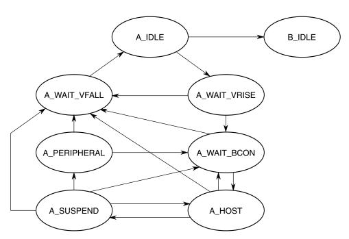
Figure 40-93. Dual role A device flow diagram
