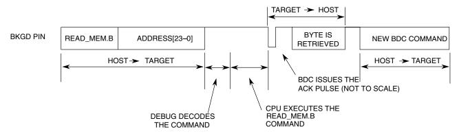
Figure 51-8. Handshake Protocol at Command Level
