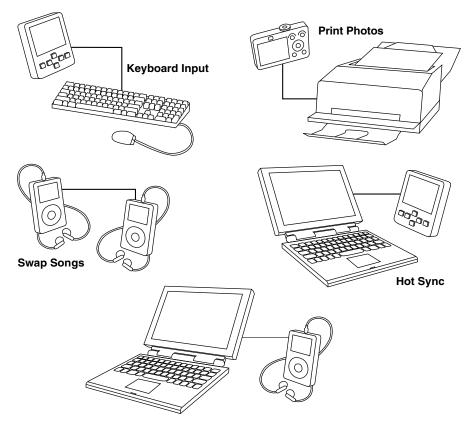
Figure 40-2. Example USB 2.0 On-The-Go configurations
