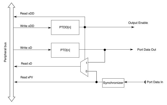
Figure 47-79. Diagram of port data logic function
