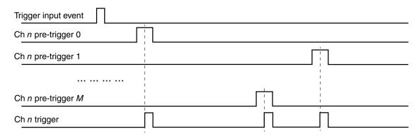
Figure 34-42. Pre-trigger and trigger outputs
