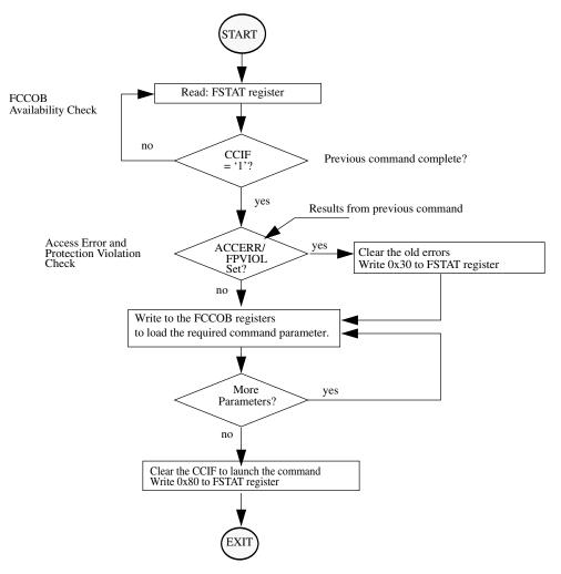
Figure 24-32. Generic Flash Command Write Sequence Flowchart
