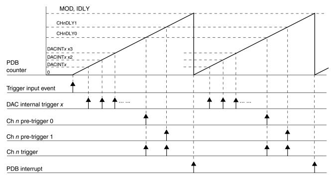
Figure 34-43. PDB ADC triggers and DAC interval triggers use case
