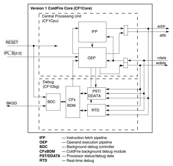
Figure 51-1. Simplified Version 1 ColdFire Core Block Diagram
