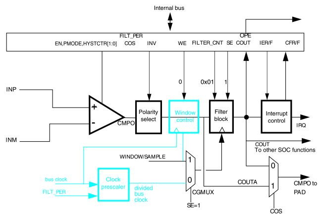
Figure 31-16. Sampled, Non-Filtered (# 3A): sampling point externally driven
