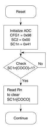
Figure 30-48. Initialization flowchart example
