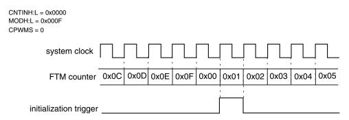
Figure 38-205. Initialization trigger is generated when the FTM counter achieves the value of CNTINH:L
