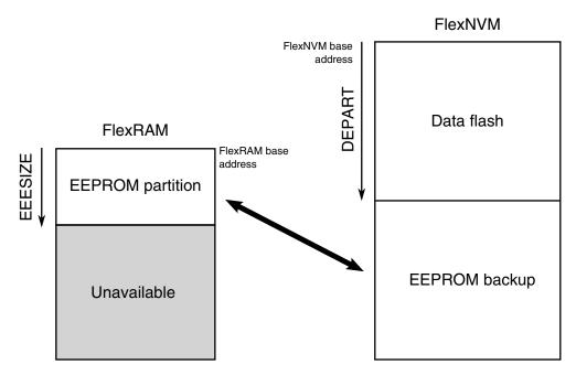
Figure 24-30. FlexRAM to FlexNVM Memory Mapping
