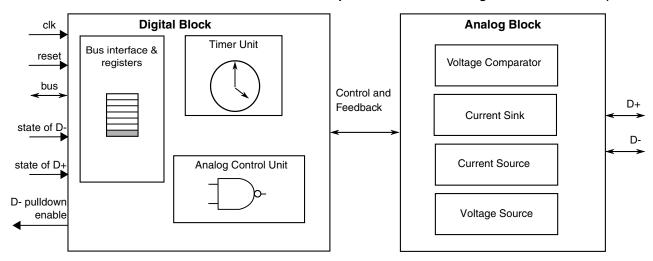
Figure 41-1. Block diagram
