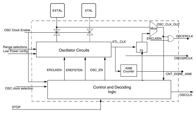
Figure 22-1. OSC Module Block Diagram
