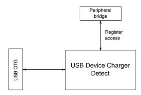
Figure 3-39. USBDCD configuration
