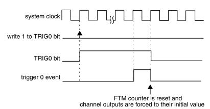
Figure 38-192. FTM counter synchronization when (REINIT = 1), (PWMSYNC = 0), and a hardware trigger was used
