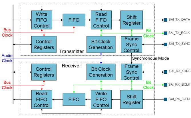
Figure 45-1. I<sup>2</sup>S/SAI block diagram
