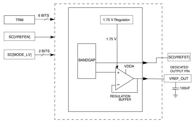
Figure 33-1. Voltage reference block diagram
