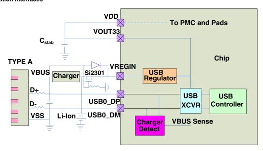
Figure 3-36. USB regulator Li-ion use case
