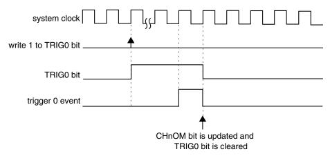
Figure 38-190. CHnOM Synchronization when (SYNCHOM = 1), (PWMSYNC = 1), and a hardware trigger was used
