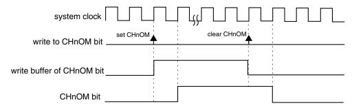
Figure 38-187. CHnOM synchronization when (SYNCHOM = 0)
