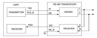
Figure 44-119. Transceiver driver enable using RTS
