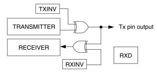
Figure 44-115. Loop operation (C1[LOOPS] = 1, C1[RSRC] = 0)
