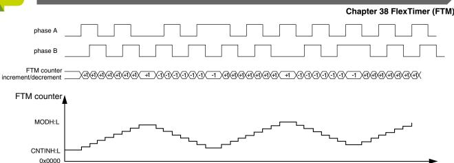
Figure 38-218. Quadrature Decoder – Phase A and Phase B Encoding Mode
