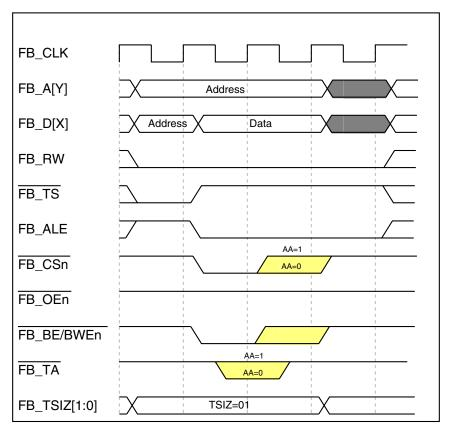
Figure 25-18. Single Byte-Write Transfer
