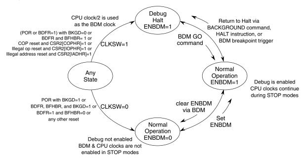
Figure 51-2. Debug Modes State Transition Diagram
