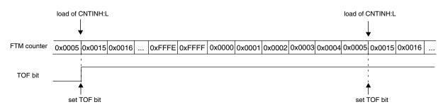
Figure 38-147. Example of up counting when the value of CNTIN registers is greater than the value of MOD registers
