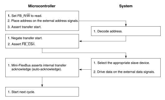
Figure 25-13. Read Cycle Flowchart
