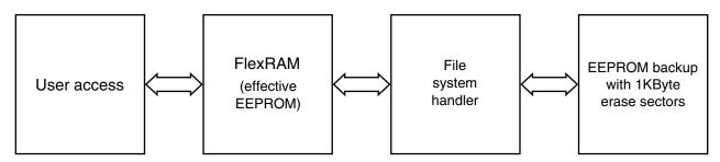
Figure 24-29. Top Level EEPROM Architecture
