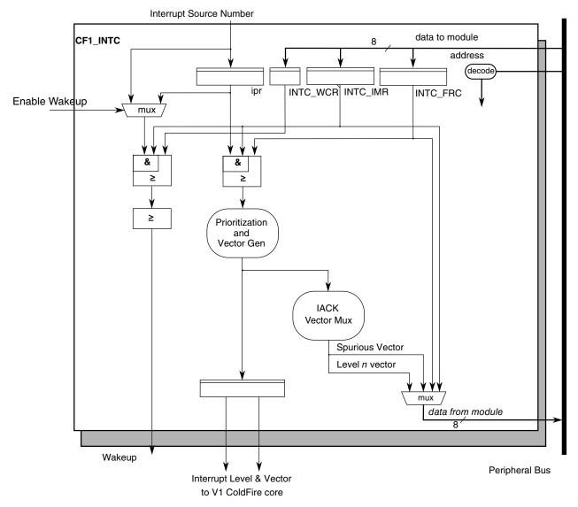
Figure 15-1. CF1\_INTC Block Diagram
