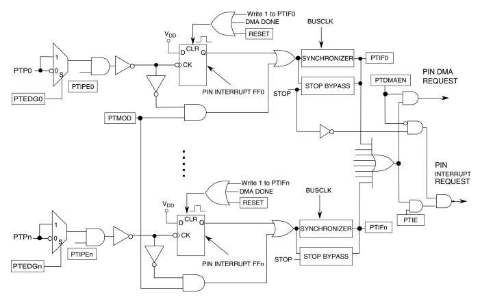
Figure 47-81. Diagram of pin interrupt function
