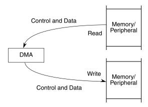
Figure 20-2. Dual-Address Transfer
