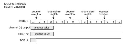
Figure 38-155. Example of the output compare mode when the match sets the channel output
