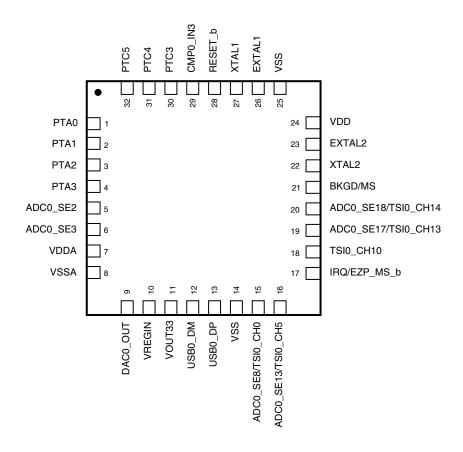
Figure 9-5. 32-pin QFN
