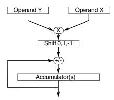
Figure 12-1. Multiply-Accumulate Functionality Diagram
