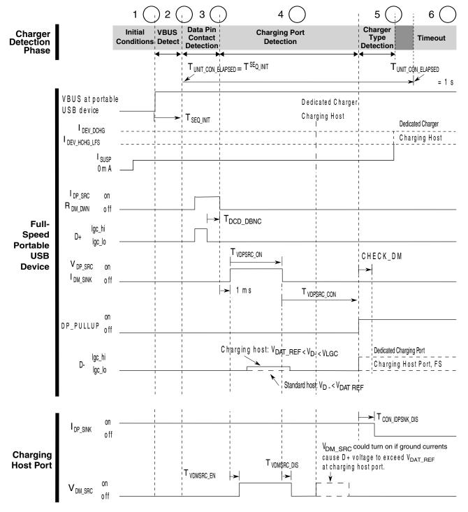
Figure 41-9. Full speed charger detection timing
