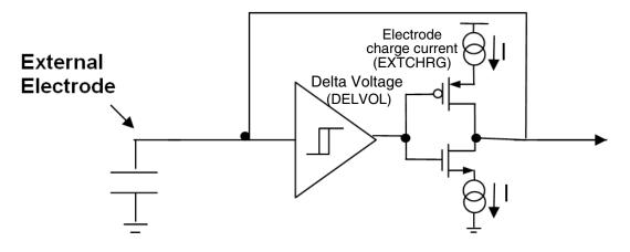
Figure 49-64. TSI electrode oscillator circuit
