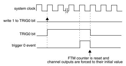
Figure 38-193. FTM counter synchronization when (REINIT = 1), (PWMSYNC = 1), and a hardware trigger was used
