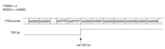
Figure 38-149. Example when the FTM counter is a free running
