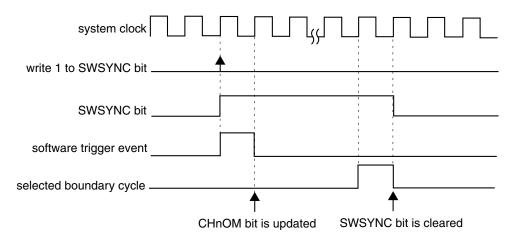
Figure 38-188. CHnOM synchronization when (SYNCHOM = 1), (PWMSYNC = 0) and software trigger was used
