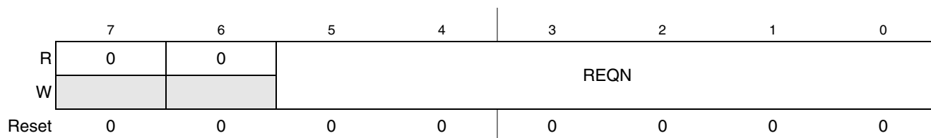
Figure 8-3. Programmable Level 6, Priority {7,6} Registers (INTC_PL6P{7,6})
