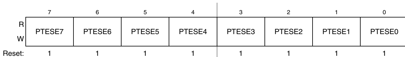
Figure 9-30. Slew Rate Enable for Port E Register (PTESE)
