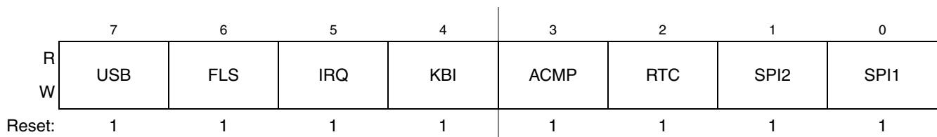
Figure 5-10. System Clock Gating Control 2 Register (SCGC2)
