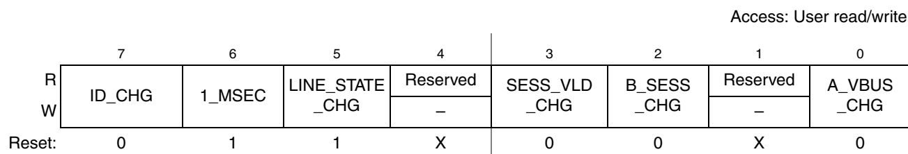
Figure 16-13. OTG Interrupt Status Register
