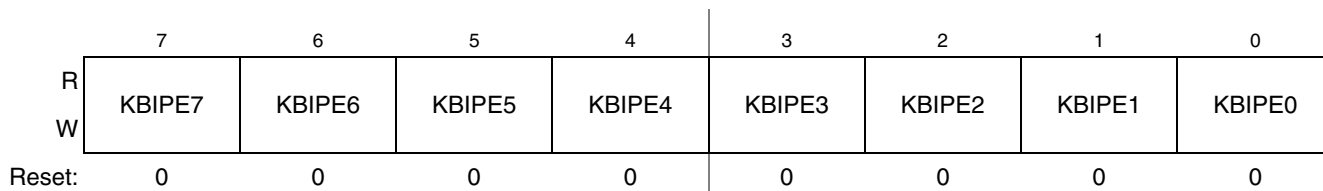
Figure 9-58. KBI1 Interrupt Pin Select Register (KBI1PE)
