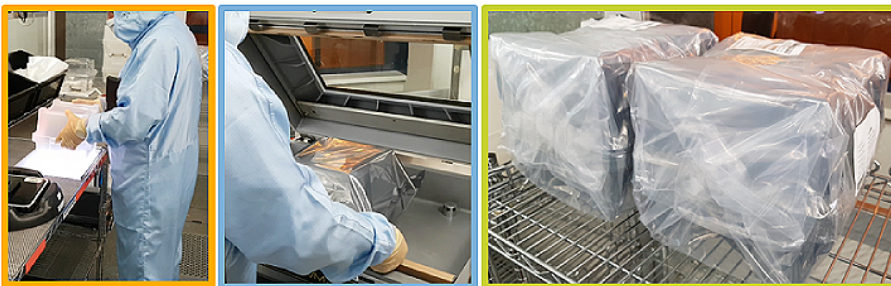
Visual check after closing transport box First: Placement of sticker Ready to be taken out of the clean room for shipment Second: Wrapping
