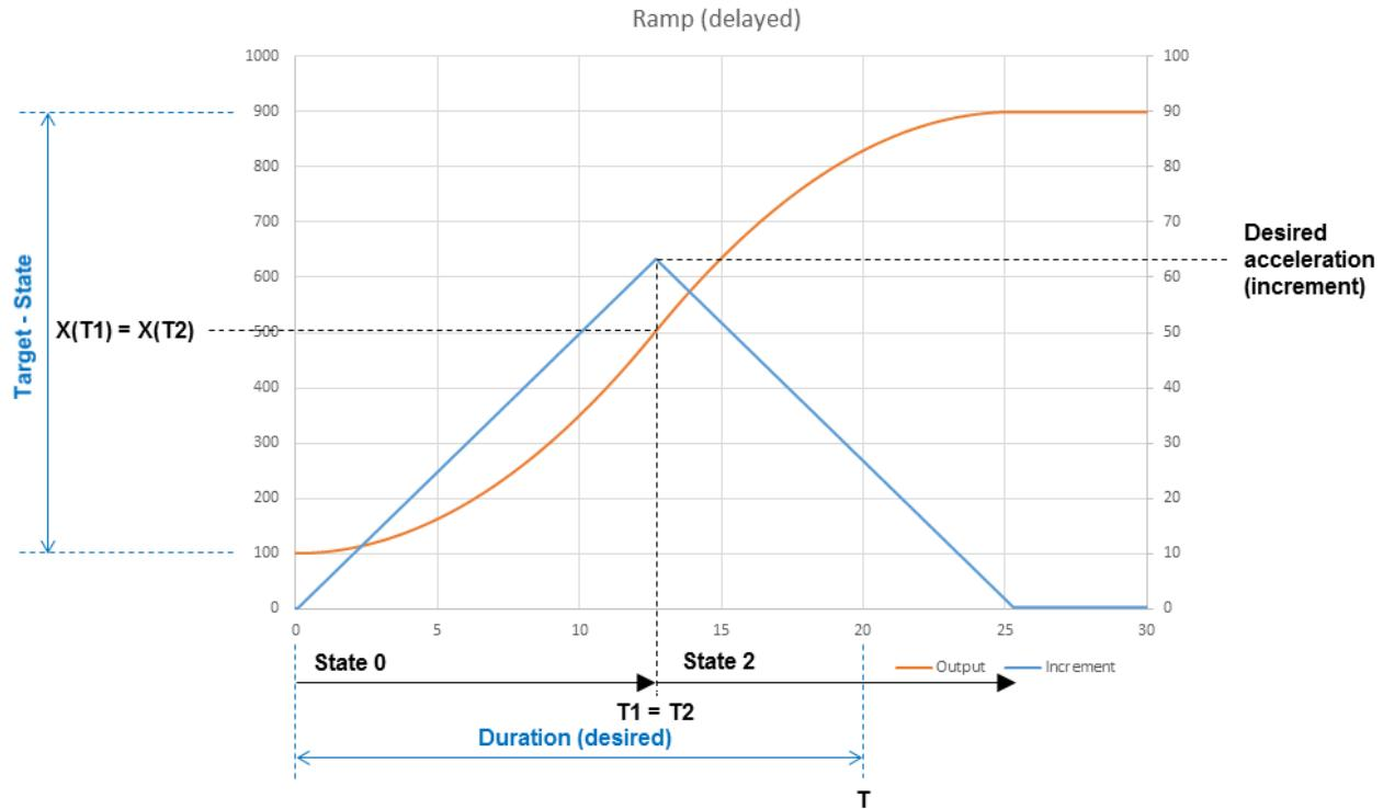
Figure 67. GFLIB\_FlexSRamp delayed profile
