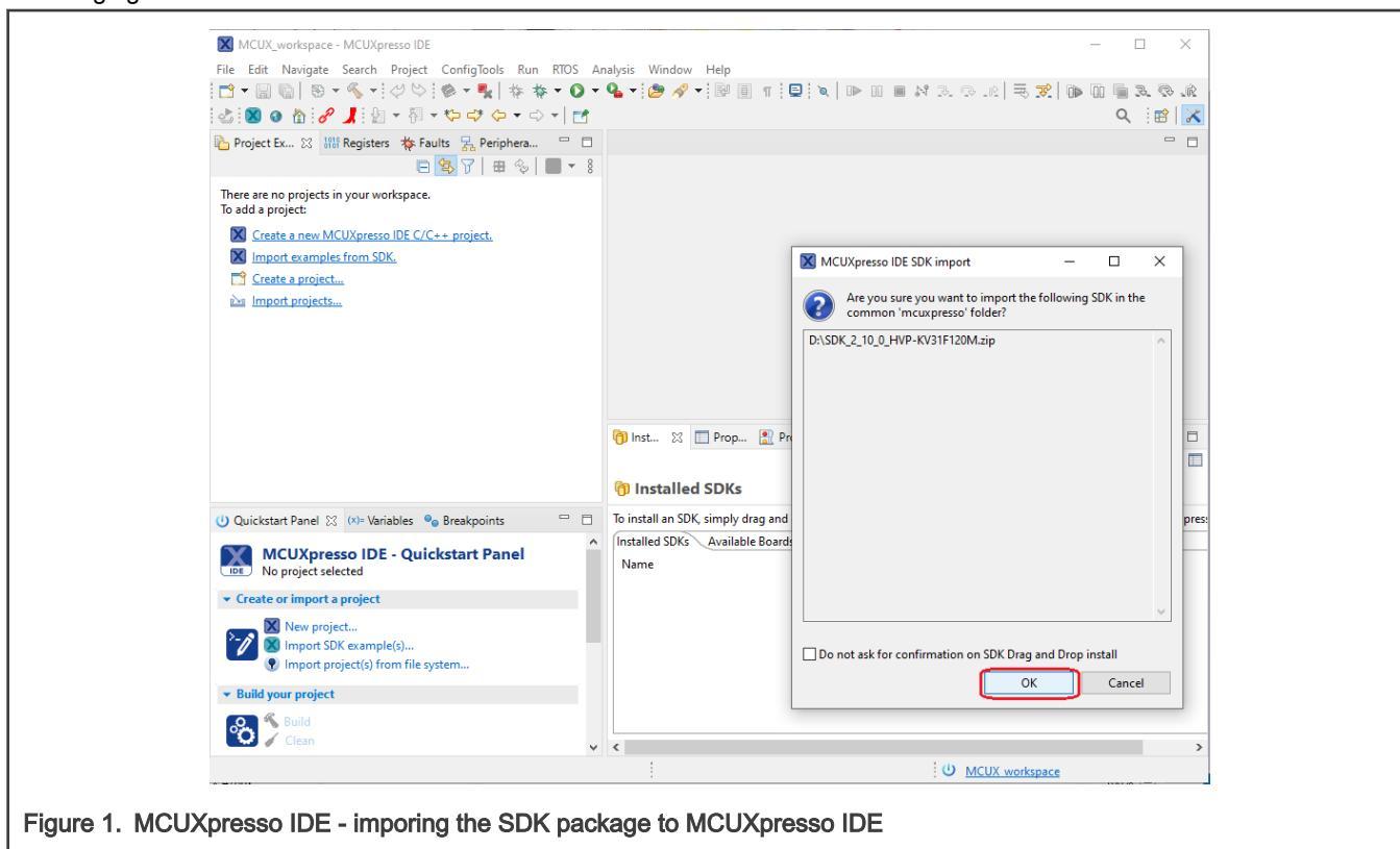
Figure 1. MCUXpresso IDE - imporing the SDK package to MCUXpresso IDE
