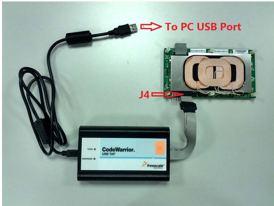
Figure 28 Connecting the debug cable to the board
