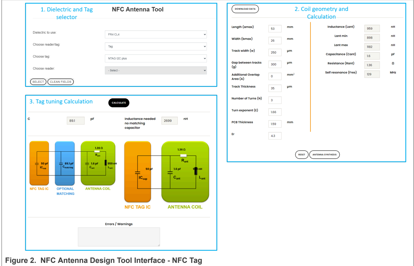
Figure 2 shows the NFC Tag Antenna and tuning calculation part.
