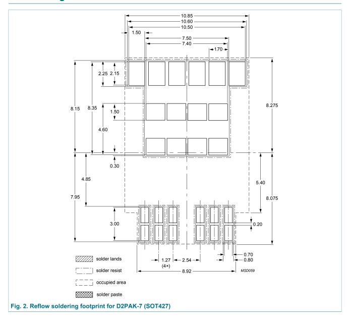
Plastic single-ended surface-mounted package (D2PAK-7); 7 leads (one lead cropped)
