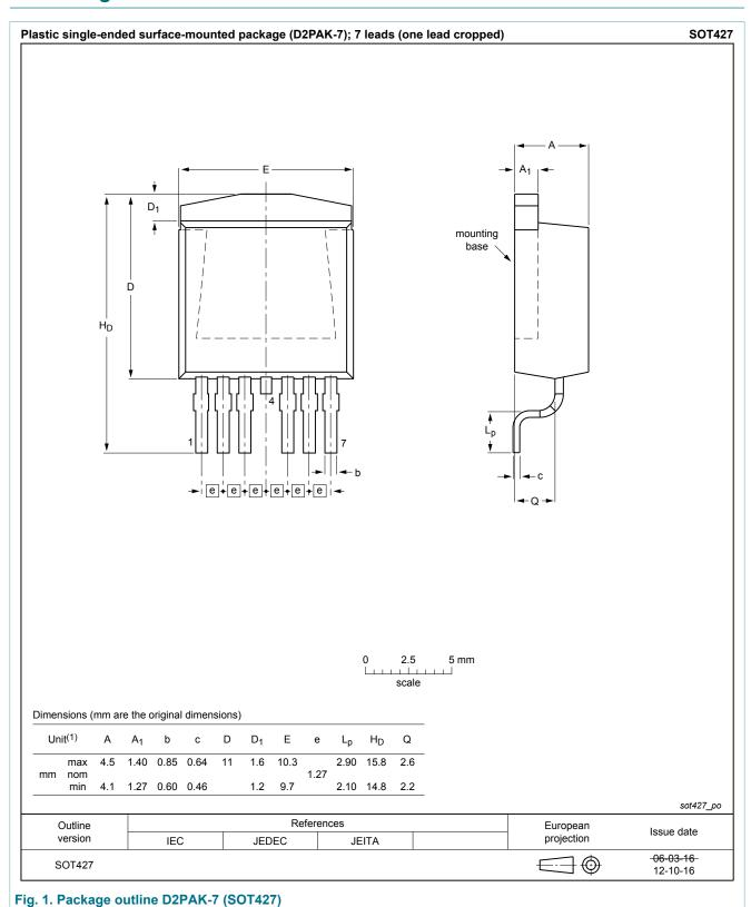
Plastic single-ended surface-mounted package (D2PAK-7); 7 leads (one lead cropped)
